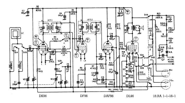
Figures in circles refer to the voltages on the various electrodes. All voltages were taken with an Avo 7 meter on the highest permissible range.
