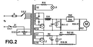
Resistors R27 and R33/37 are connected in parallel to the measuring instrument to match it to the series resistors R44 and R43. Checking of card 1C is necessary every now and then to test if the rectifier valve L1 is working properly after the line voltage has been adjusted. A deviation of up to five scale marks is allowed.
