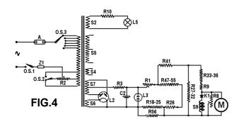
The current through the measuring instrument is adjusted by R8 so that it, together with K1-S9 and R8 parallel to the instrument, is exactly 0.1mA. The first 100° are marked red. When used for measuring the emission of a valve this range shows the limit of the usefulness of valve checked. K1-S9 are for the following reasons connected in parallel to the measuring instrument....
