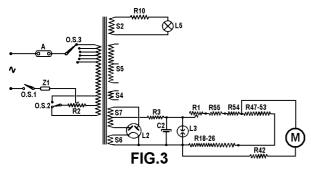
R42 serves as a dropping resistor for the  $\mu A$  meter used as a voltmeter. The meter can be adjusted to full deflection by changing R1. The current flowing through the potentiometer R1-R47/55-R18/26 is exactly 10mA. The voltages across each resistor are therefore exactly defined. This potentiometer is later used to obtain the negative grid voltage for the valve to be checked.
