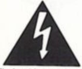
The lightning flash with arrowhead, within an equilateral triangle, is intended to alert the user of the presence of uninsulated "dangerous voltage" within the product's enclosure that may be of sufficient magnitude to constitute a risk of electric shock to persons.
