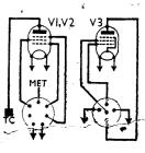
Circuit diagram of the Philips 821B. R12 shunts the GB section of the HT battery via S7. The Droitwich rejector L1, C16 is in circuit only in the fourth switch position.
