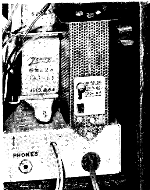
Figure 4.—Ballast Adaptor Inserted in Socket.
