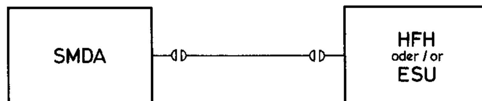
Fig. 3-4 Test setup for harmonics measurement
