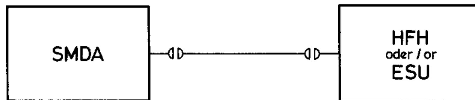
Fig. 3-4 Test setup for harmonics measurement
