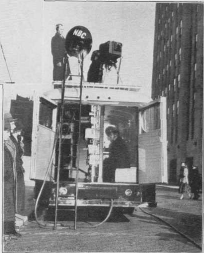
FIG. 40. A PLATFORM ON THE TOP OF THE PICK-UP UNIT OFFERS A POINT OF VANTAGE FOR THE CAMERA AND MICROPHONE. THE MONITORING OPERATOR CAN BE SEEN AT THE CONTROLS IN THE VAN. SPACE IS PROVIDED ON THE LEFT FOR THE CAMERA AND THE REELS OF COAXIAL CABLE REQUIRED FOR CONNECTIONS WHICH RUN OUT FROM THE TERMINALS BELOW THE DOORS.
