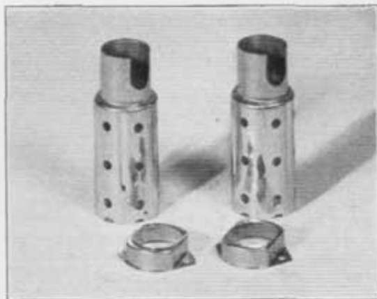
FIG. 51. TWO OF THE GLASS TUBES REQUIRE THE METAL SHIELDS SHOWN HERE. THE BASES ARE MOUNTED ON THE CHASSIS IN ASSEMBLY STAGE NO. 1, BUT THE SHIELDS ARE NOT PUT IN PLACE UNTIL THE TUBES ARE
