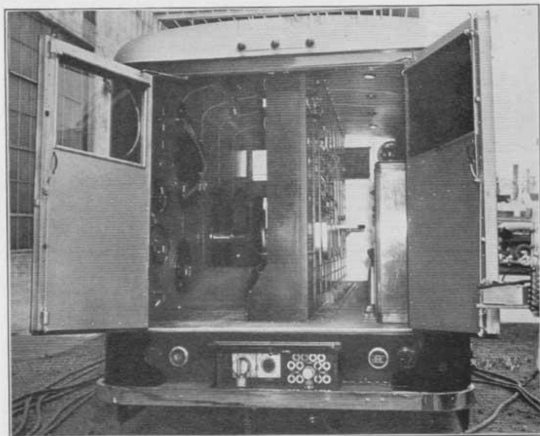
FIG. 38. INTERIOR OF THE PICK-UP UNIT OF THE MOBILE EQUIPMENT. THIS CONTAINS THE VIDEO AMPLIFIER AND MONITORING CONTROLS.
