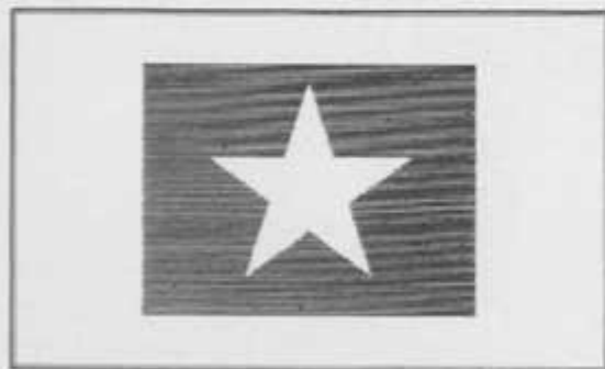
FIG. 18. THE COMPLETED FRAME, COMPRISING THE FIRST INTERLACE, FOLLOWED BY THE SECOND INTERLACE SCANNING.
