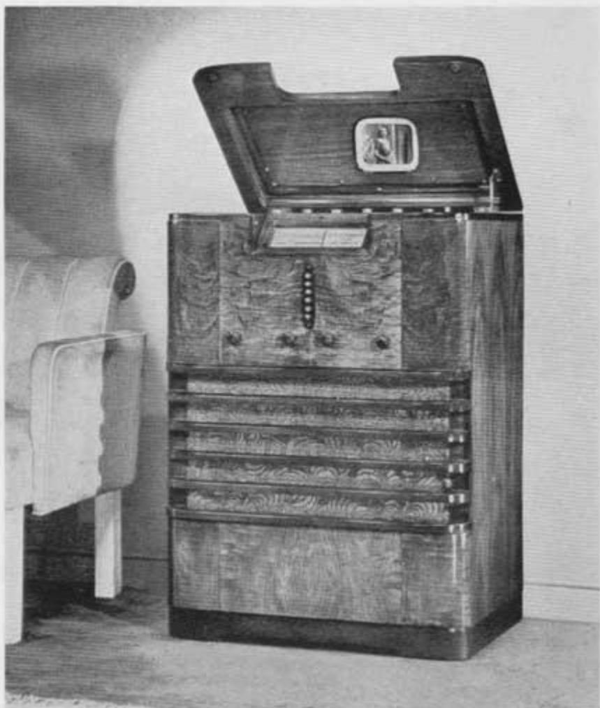
FIG. 24. THE ANDREA KT-E-5 CHASSIS CAN BE MOUNTED IN THIS MANNER FOR MIRROR VIEWING. CONTROLS AT THE TOP ARE FOR THE TELEVISION SET, AND AT THE FRONT, FOR AN ALL-WAVE SOUND RECEIVER. THIS MAKES A MOST ATTRACTIVE PIECE OF FURNITURE.
