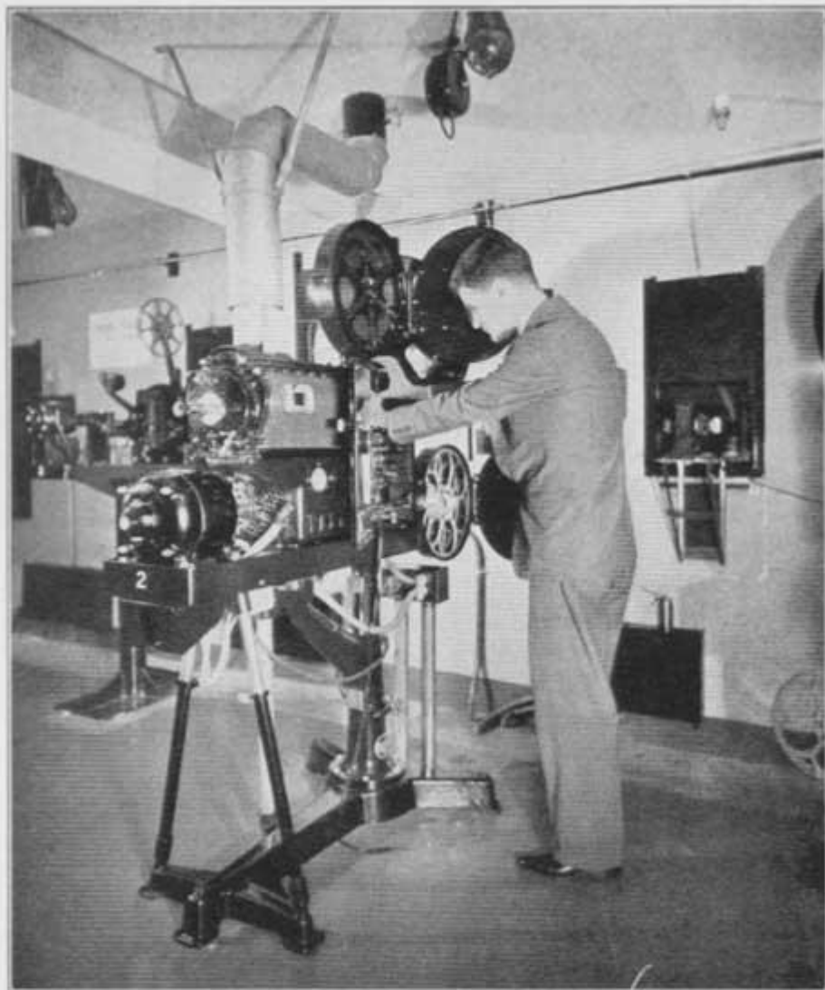
FIG. 23. ANOTHER PIECE OF NBC STUDIO EQUIPMENT. THIS IS THE MACHINE WHICH PROJECTS FILM INTO THE CAMERA, FOR TRANSMITTING MOVIES. THERE IS LESS FLICKER AT THE TELEVISION PICTURE TUBE THAN WHEN FILM IS SEEN ON THE SCREEN IN A THEATRE.
