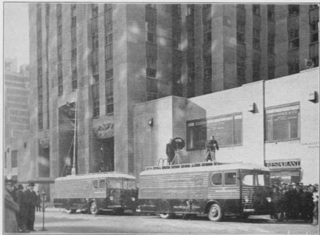
FIG. 21. THIS IS THE NBC EQUIPMENT USED FOR SPOT NEWS EVENTS, SUCH AS TELEVISIONING THE ENGLISH KING AND QUEEN DURING THEIR VISIT TO NEW YORK CITY, AND THE NOVA-BAER FIGHT. PROGRAMS ARE SENT TO THE EMPIRE STATE BUILDING, AND REBROADCAST ON 44-50 MC.
