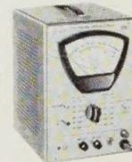
**A 403 A** • Wide range Millivoltmeter • DC range: 1 mV to 300 V (fsd) 12 scales • Frequency range: 5 cps to 2 Mc.
