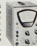
**AG 201** • VSWR Indicator, suitable with wave guide or coaxial slotted sections • Operating frequency: 1000 cps ( $\pm 5\%$ ) • Sensitivity: 0.2  $\mu$ V (fsd) • Crystal rectifier or bolometer or high impedance inputs • 5 measurement scales in VSWR and dB • Band spread dB scale • Range: 70 dB.
