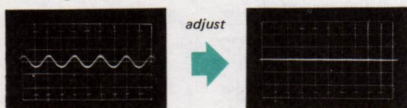
Fig. 3-6. Fm discriminator alignment output response
