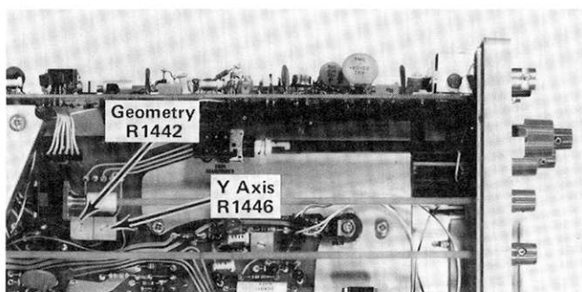
Fig. 5-5. Location of Geometry and Y Axis adjustments.
