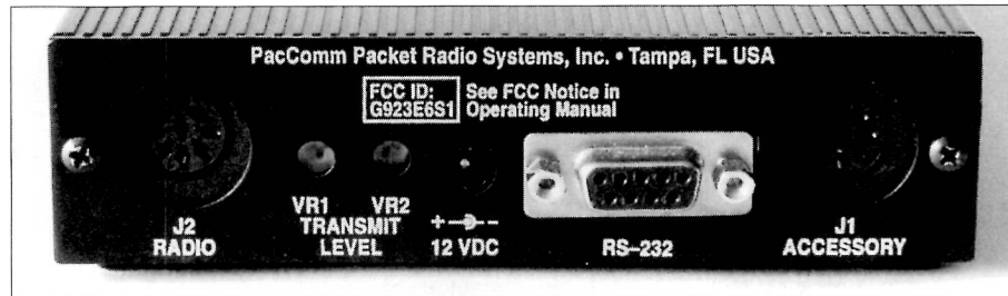
Fig 7.9. Rear-panel connections on the TNC interface to your radio and RS-232 terminal
