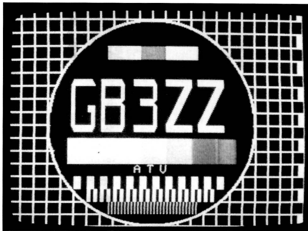
Fig 8.5. Off-air capture of the Bristol 24cm repeater test card over 25km distance
