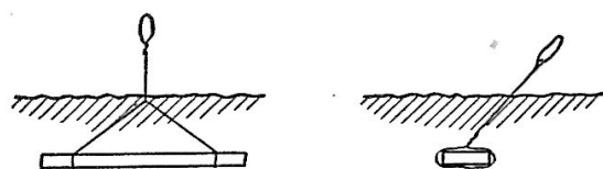
Fig. 1613 — The "dead man" guy anchor.
