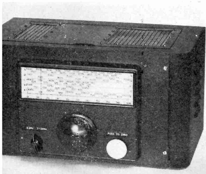
Fig. 6-84—The v.f.o. unit mounted in its cabinet. Holes are drilled in the dial cover to accommodate the switch shafts. At the right, a poker chip has been cemented to the v.f.o. set push-button switch so that it can be operated while tuning the v.f.o.; this makes frequency-spotting a one-handed operation.
