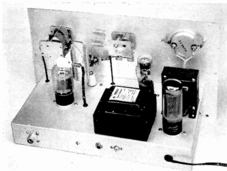
Fig. 6-37—Rear view of the transmitter showing the placement of components above chassis. The loading capacitor, C_8 , is at the left, L_3 is the vertical coil and L_2 the horizontal one. Rubber grommets are used to prevent chafing and to furnish additional insulation on the leads coming from below chassis.
