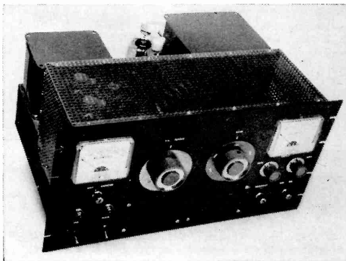
Fig. 6-67—This amplifier operates at a plate input of approximately 500 watts, uses a pair of 811As in grounded-grid, and is complete with power supply on a 13 \times 17 \times 4 -inch chassis. The rack panel is 10\frac{1}{2} by 19 inches. Front-panel controls include the plate tuning capacitor and band switch in the center, filament and plate power switches with their pilot lights at the lower left, sensitivity control and forward-reflected power switch for the directional coupler at the lower right, variable loading capacitor and auxiliary loading-capacitor switch underneath the 0-1 milliammeter at the right, and the grid-cathode milliammeter with its switch at the upper left. The filter choke, 866As and plate transformer occupy the rear section of the chassis.
