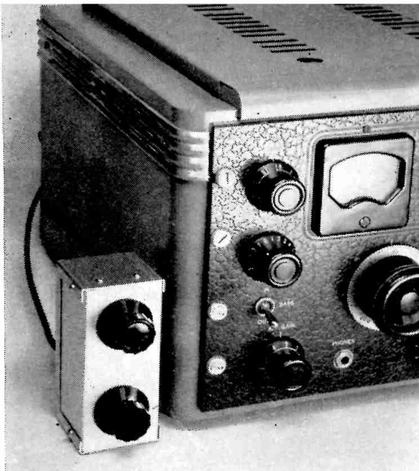
Fig. 5-63—View of the Q multiplier showing its single connecting cable to the receiver. The box can be placed in any convenient spot on or around the receiver.
