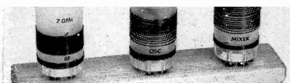
Fig. 5-59—Each set of coils is provided with a wooden base for storage. C_2 and C_4 are mounted in the recesses at the tops of the oscillator and mixer coil forms.
