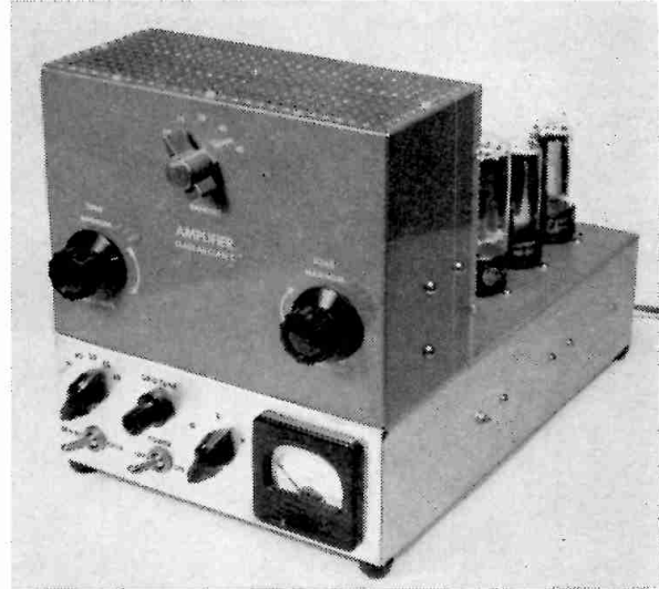
Fig. 6-47—Front view of the 6146 all-purpose amplifier. The upper panel is part of an 8 \times 6 \times 3\frac{1}{2} -inch Minibox (Bud CU-2109); the ventilated shielding of Reynolds Aluminum cane metal is fastened to the Minibox and base with sheet-metal screws.
