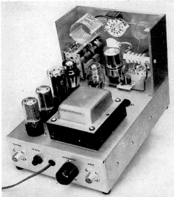
Fig. 6-48—Rear view of the 90-watt all-purpose amplifier with the cane-metal cover removed. One voltage-regulator tube has been removed from its socket (right edge of transformer) to allow the neutralizing capacitor and plate blocking capacitor to be seen. The plate r.f. choke (RFC 3 in Fig. 6-49) is mounted on one side wall, and the load capacitor and safety choke ( C_4 and RFC 4 in Fig. 6-49) are mounted on the far side wall.
