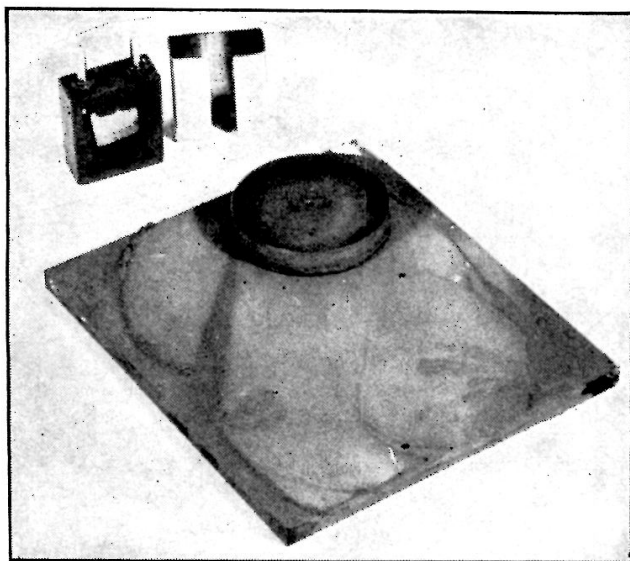
Fig. 6-7 — The equipment necessary for grinding a crystal blank to frequency. A piece of plate glass and a "button" of the same material are essential. The "quick-change" adaptation for the crystal holder is a convenience. Not shown, but also convenient, are a small paint brush for spreading abrasive and a toothbrush for scrubbing.
