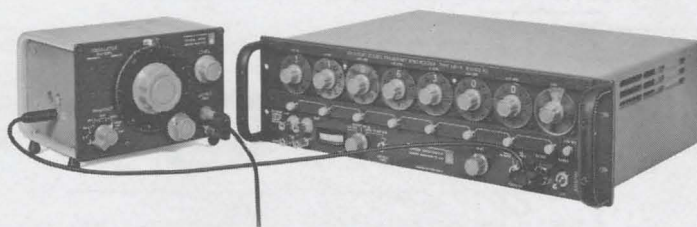
Figure 4-3. The Type 1309 Oscillator being synchronized with the Type 1161-A7C Coherent Decade Frequency Synthesizer.
