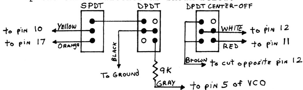
2. Isolate pin 10 of the MB8719 chip. Solder Yellow wire to pin 10.
