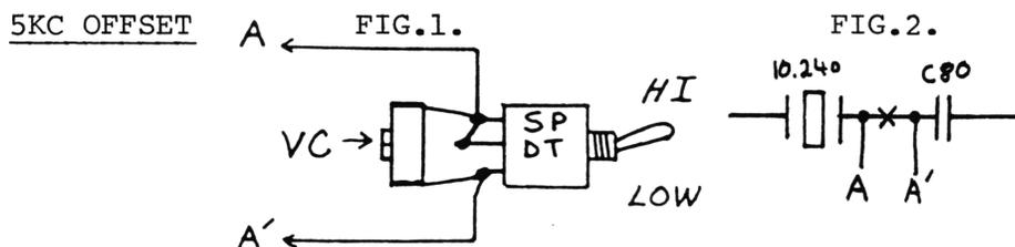
1. Wire up the SPDT switch and trim capacitor as shown in Fig.1.
