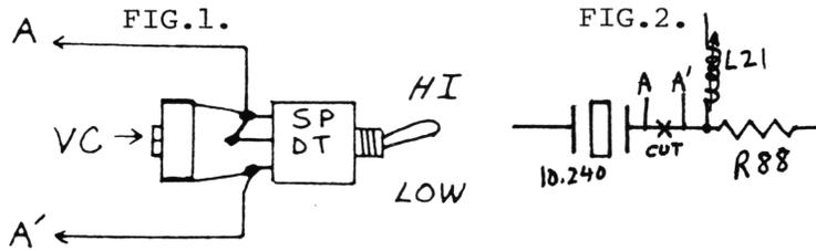
1. Wire up the SPDT switch and trim capacitor as shown in Fig.1.
