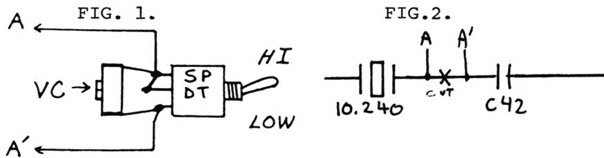
1. Wire up the SPDT switch and trim capacitor (supplied) as shown in Fig. 1.
