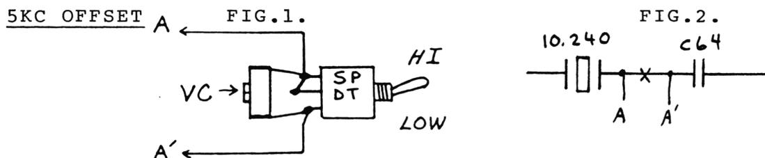
1. Wire up the SPDT switch and trim capacitor as shown in Fig.1.
