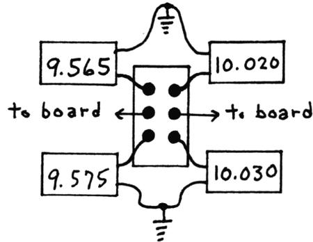
MIKE WIRING: 4 Pin Locking Ring Connector - Relay Switching.
