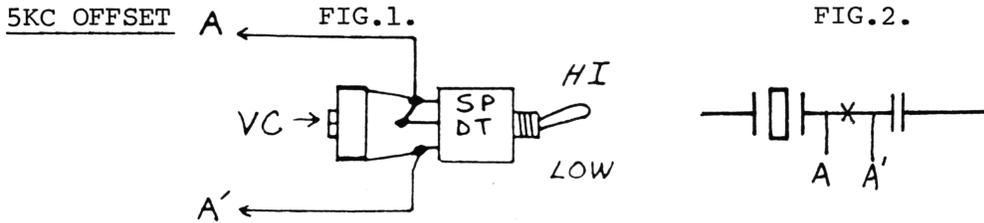
1. Wire up the SPDT switch and the trim capacitor as shown in Fig.1.
