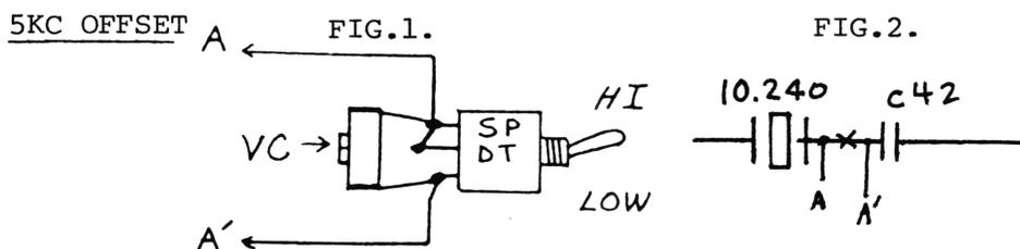
1. Wire up the SPDT switch and trim cap as shown in Fig.1.
