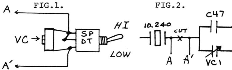
1. Wire up the SPDT switch and trim cap as shown in Fig.1.
