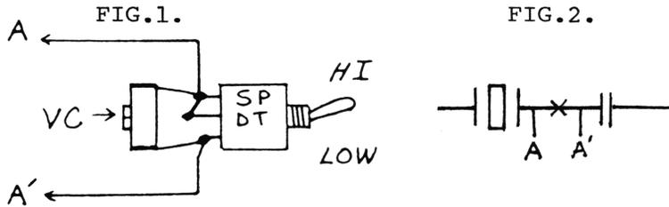
1. Wire up the SPDT switch and trim capacitor as shown in Fig.1.
