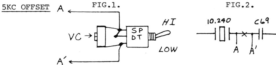
1. Wire up the SPDT switch and trim capacitor as shown in Fig.1.
