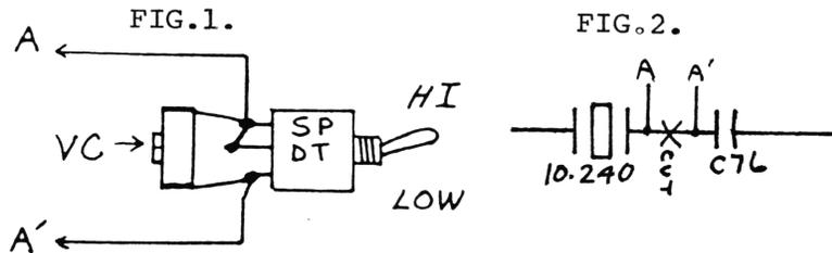
1. Wire up the SPDT switch and the trimmer capacitor (supplied) as shown in Fig.1.
