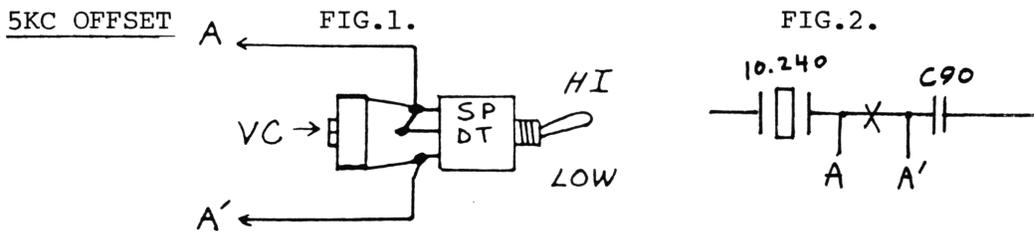
1. Wire up the SPDT switch and trim capacitor as shown in Fig.1.
