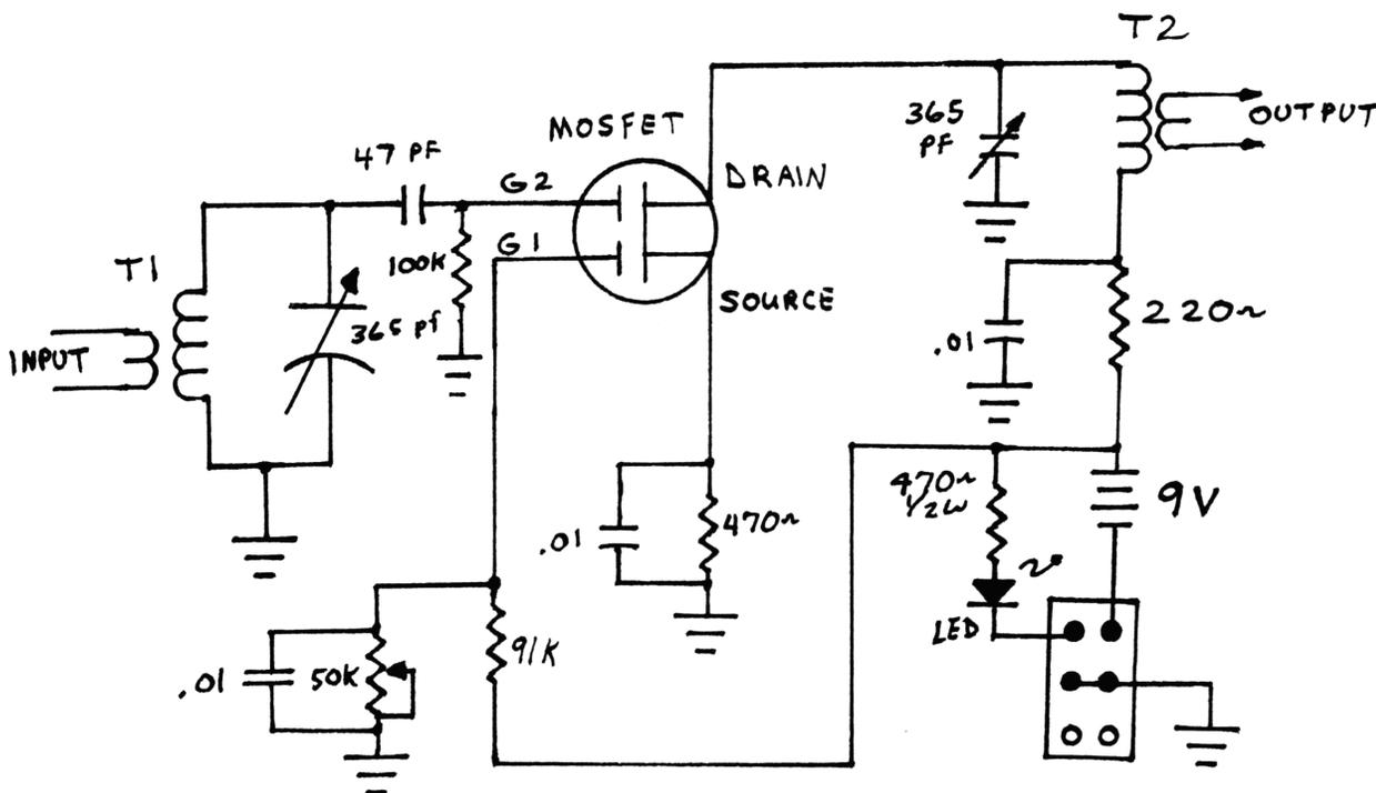
Coils should be shielded with Miller type S-33 Shields.
