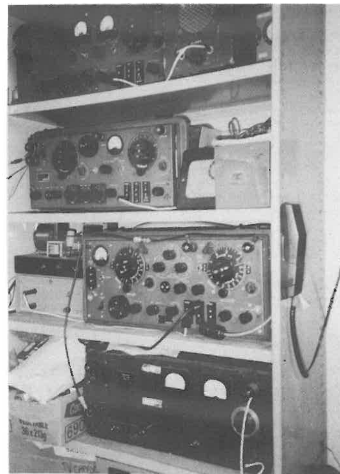
A shelf of ZC1's in George McLean's ham shack. On the top shelf is a Mk I 1st version. Second shelf a Mk I 3rd version. Third shelf a Mk II and below that a ZA1 Mk II RF Amplifier. Note the ZC1's run on a 12 volt car battery with original power supplies.
