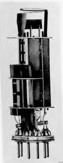
Fig. 4. The electrode system of the ECL86 triode-power pentode clearly showing the different lengths of the triode and the pentode sections. Note also the screening on the top of the triode section.
