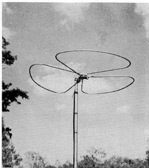
Fig. 9-43—The Big Wheel, an omnidirectional horizontal antenna for the 144-Mc. band designed by W1FVY and W1IJD. Radiating elements occupy an area approximately 40 inches in diameter.
