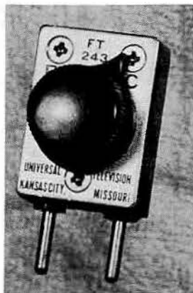
Fig. 13-2—An FT-243 surplus crystal, modified for variable frequency control.
