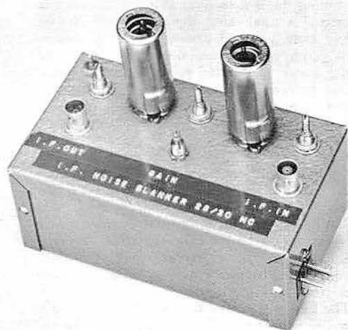
Fig. 4-47—A noise blander for insertion between a v.h.f. or u.h.f. converter and the following communications receiver. Model shown is set up for 28 to 30 Mc., but other converter output frequencies could be used by altering circuit constants.
