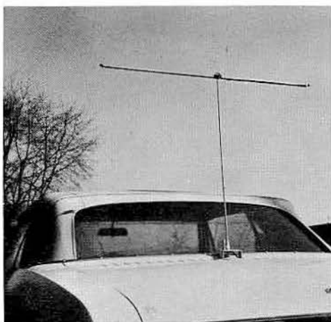
Fig. 9-57—Horizontal dipole for 2-meter mobile. The vertical support is \frac{1}{4} -inch tubing, with small coax inside, thus serving as a 1:1 balun.
