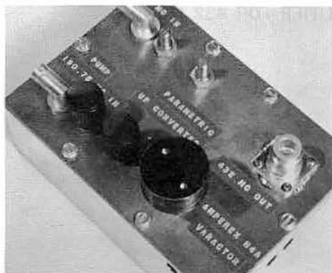
Fig. 10-29—Parametric up-converter for transferring a 50-Mc. s.s.b. signal to 432 Mc. The large black object, a heat-dissipating cap for the varactor, taken from a 2C39A tube, is not needed if an all-metal chassis is used.
