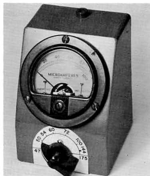
Fig. 11-7—A field-strength indicator and wavemeter for 50 and 144 Mc. The coil size is set so that the tuning range is approximately 47 to 175 Mc.
