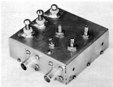
Fig. 10-24—Varactor multiplier for 1296-Mc. output with 432-Mc. drive, designed and built by W1WID. Case is a 3\frac{1}{2} by 1-inch brass box. Large screws at the left are the movable elements of capacitors C_4 , C_5 and C_7 .
