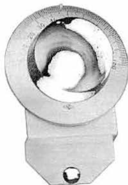
Fig. 3-6—Typical mounting for a vernier dial to be used on a general-coverage receiver. Mechanical arrangements can be worked out to fit most receivers without the necessity for drilling holes or otherwise permanently disfiguring the receiver. Adjacent control shafts and nuts provide convenient anchorages.
