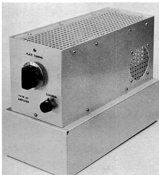
Fig. 6-33—The 829-B amplifier, with its shield cover in place. Air circulation is provided by the screened holes and cover.
