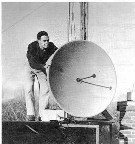
Fig. 10-52—W2BVU lines up his rooftop dish for a 2300-Mc. test beyond the visual horizon. Transmitter r.f. unit is in the weather-proof box at his feet. Reliable operating range approaches that on 144 Mc.
