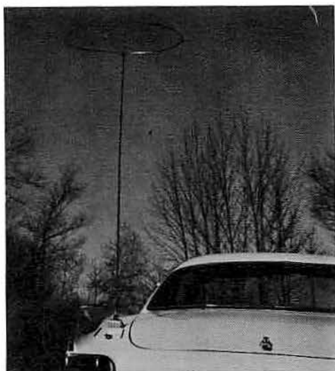
Fig. 9-53—This 144-Mc. halo appears to have no transmission line or matching device. Attached off-center to the whip of Fig. 9-52, it uses the whip as a single-wire transmission line. Optimum whip length is approximately 40 inches, so top section is telescoped when the halo is used. Very little vertical polarization is in evidence.
