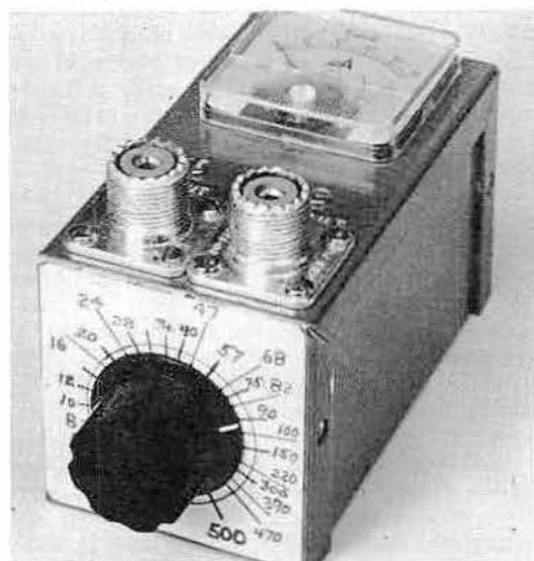
Fig. 11-16—Simple v.h.f. impedance bridge. Settings of the variable control, marked on the front of the case, represent values of impedance corresponding to nulls in meter indication.
