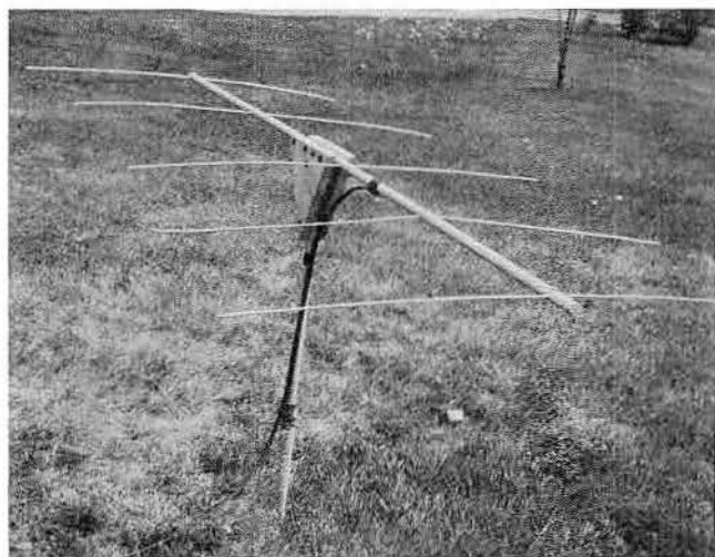
Fig. 9-29—Low-cost 5-element beam for 144 Mc. Note feedline taped to the boom and support.
