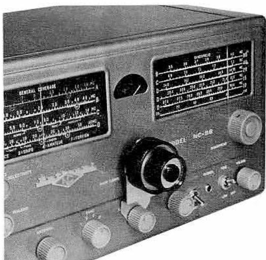
Fig. 3-7—Example of use of a two-speed planetary mechanism to slow down the tuning rate on the general-coverage dial of an inexpensive communications receiver.
