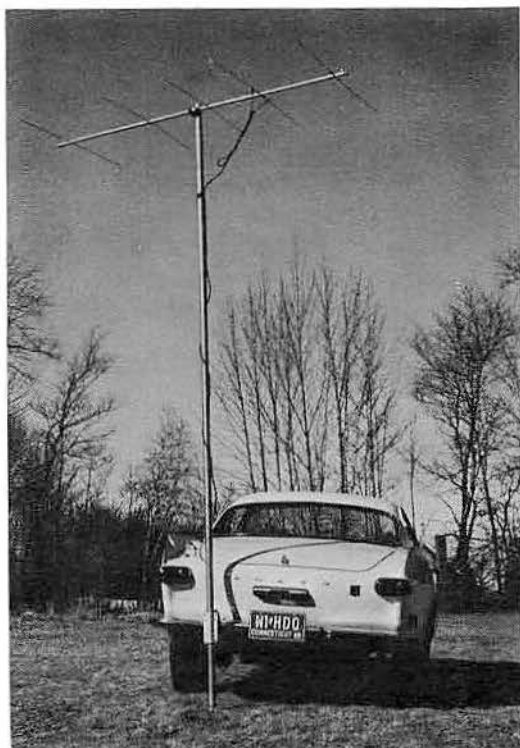
Fig. 9-58—Portable beam set up for 144 Mc., using the bumper bracket of Fig. 9-51.
