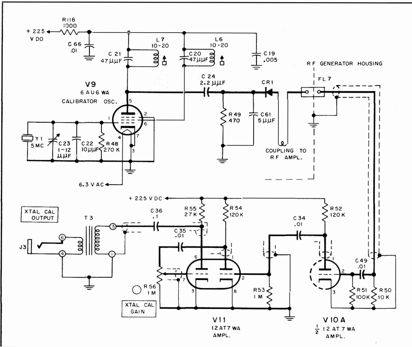
Figure 4-7. Schematic Diagram of Crystal Controlled Frequency Calibrator
