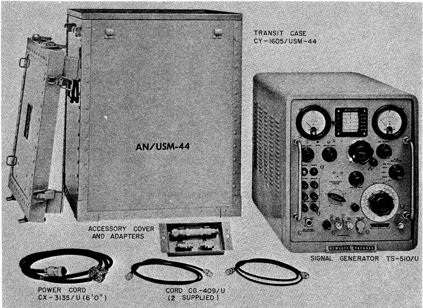
Figure 1-1. Signal Generator AN/USM-44 (Hewlett-Packard), Equipment Supplied
