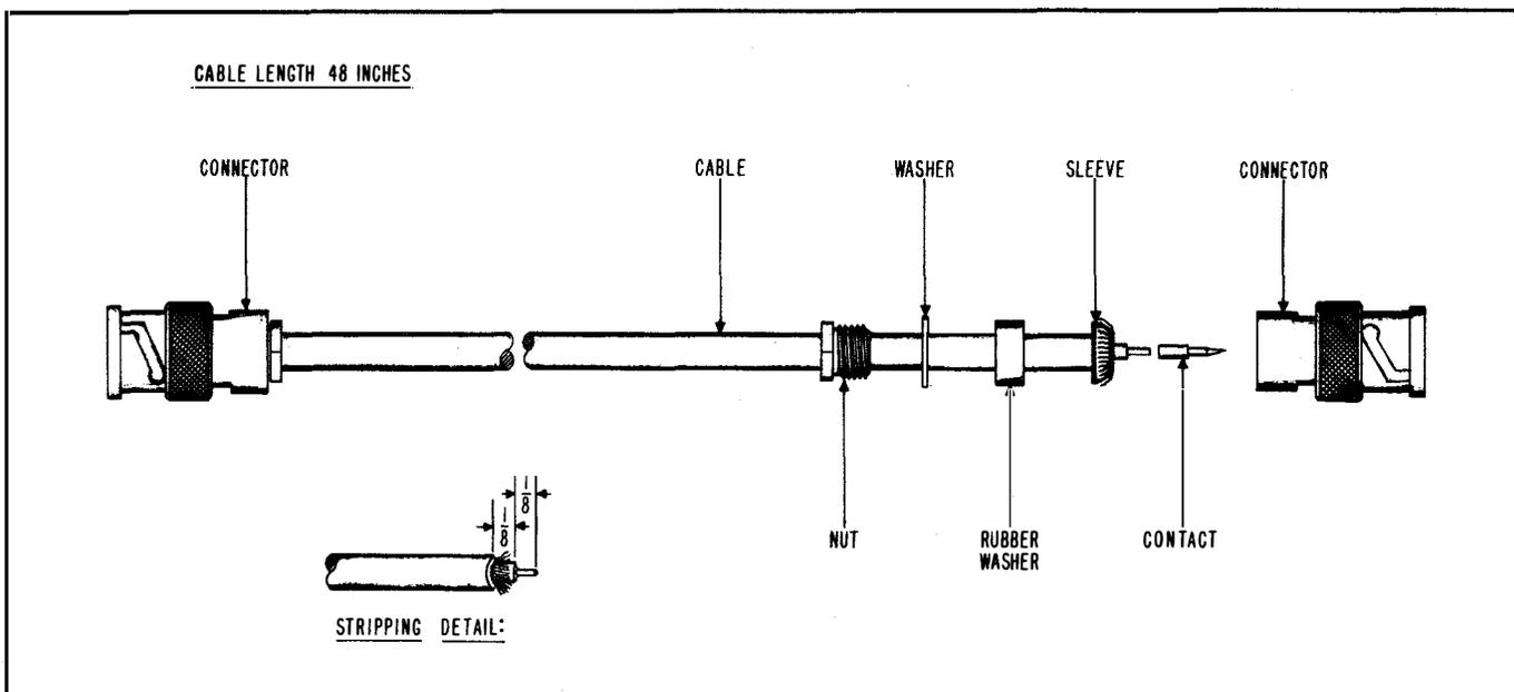
Figure 2-1. Fabrication of Video Cord CG-409/U
