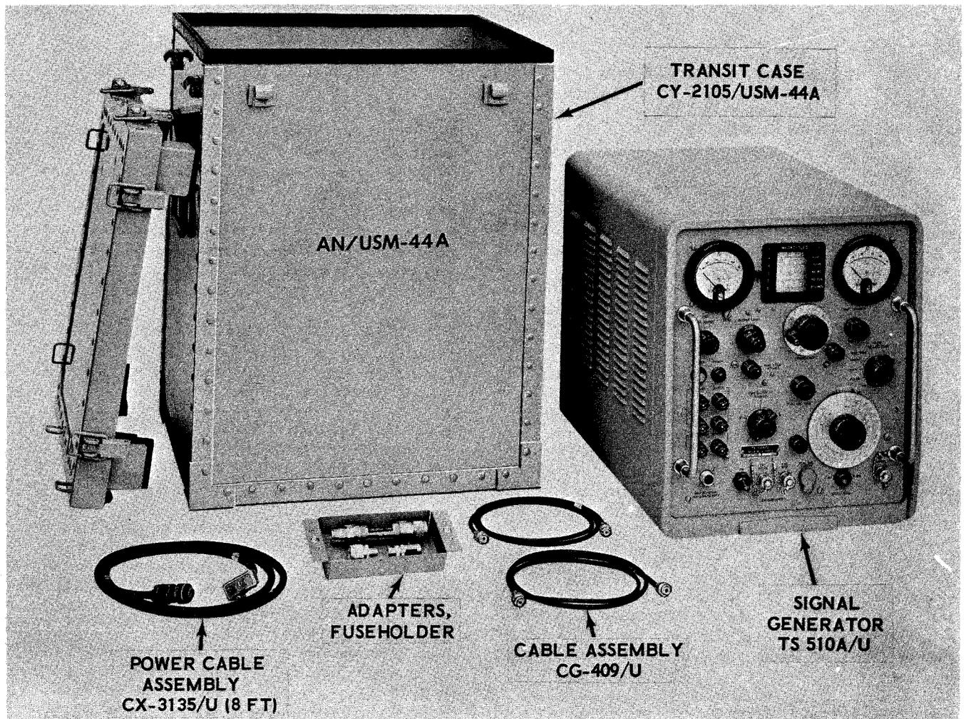
Figure 1-1A. Signal Generator AN/USM-44A (Hewlett-Packard), Equipment Supplied
