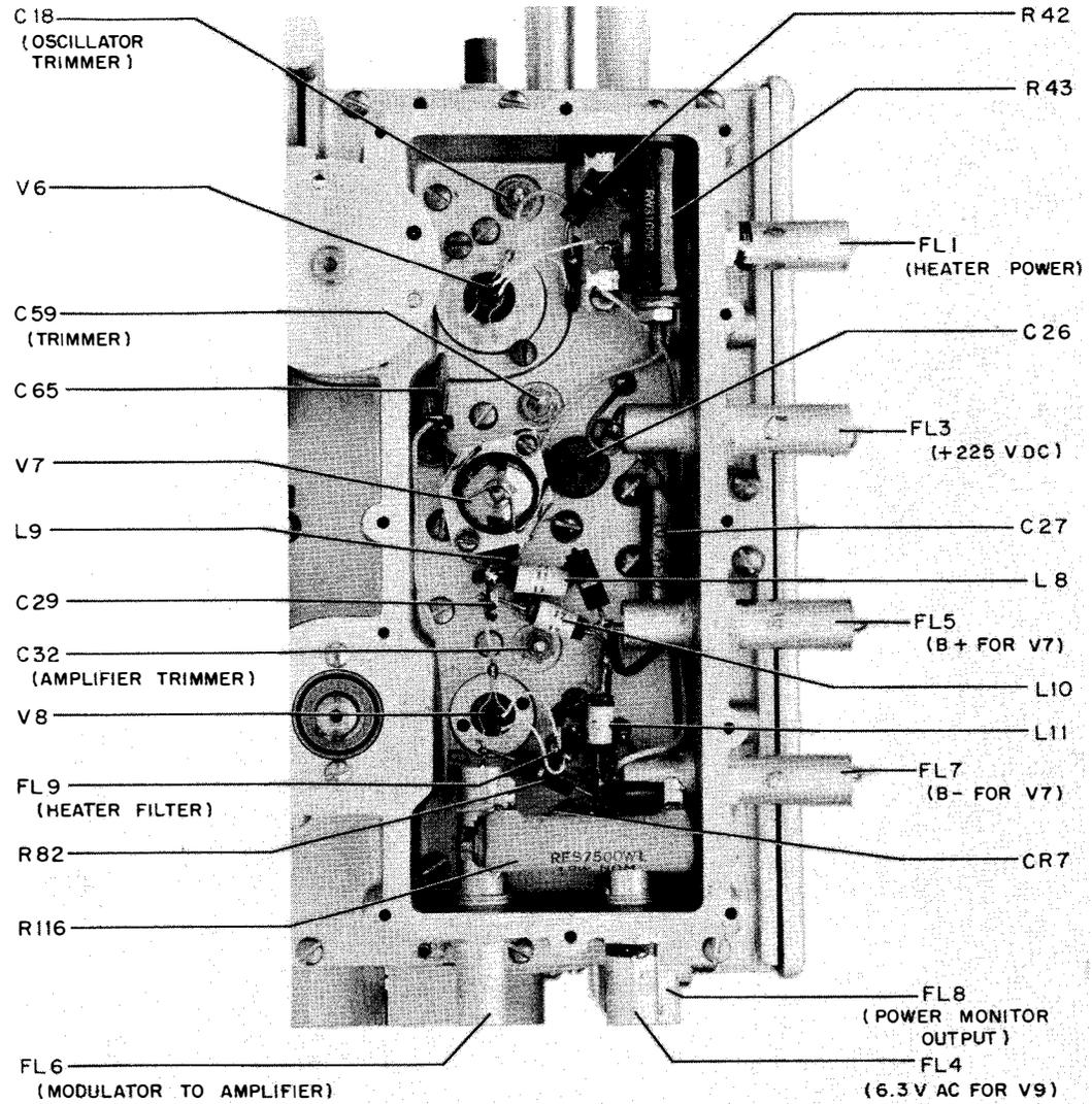
Figure 7-3. R-F Generator Assembly, Inside View of Tube Compartment
