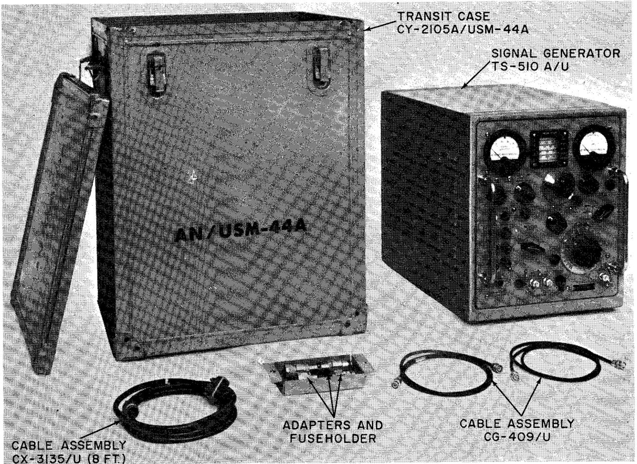
Figure 1-1C. Signal Generator AN/USM-44A (Jetric Industries), Equipment Supplied
