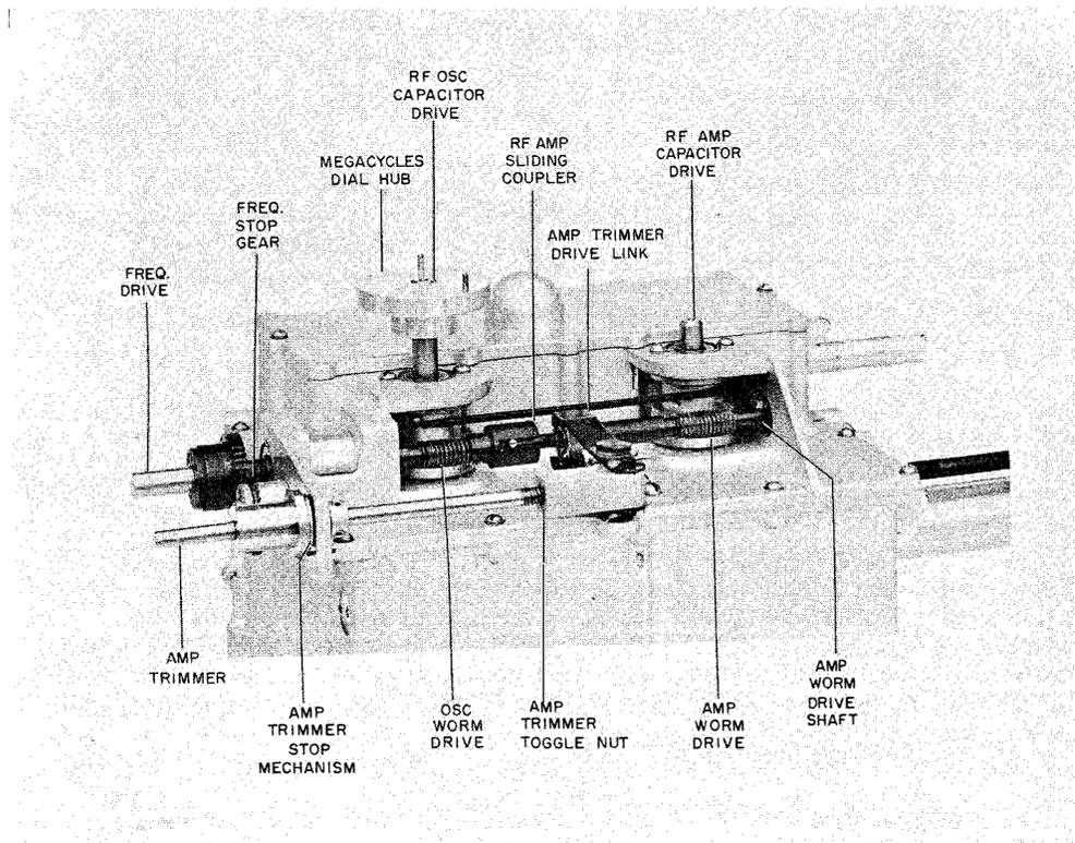
Figure 5-5. Frequency Drive Mechanism Showing Points of Lubrication
