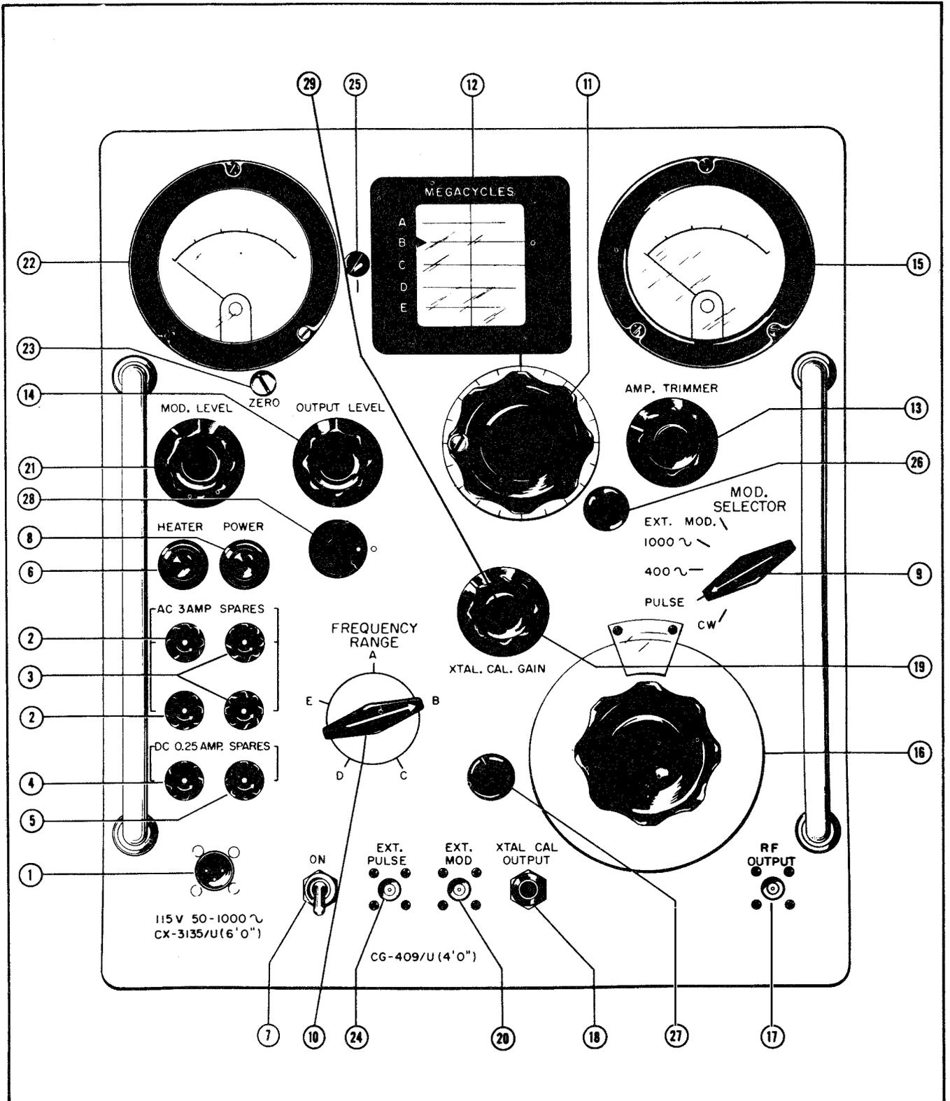
Figure 1-3. Signal Generator TS-510/U, Front Panel Controls
