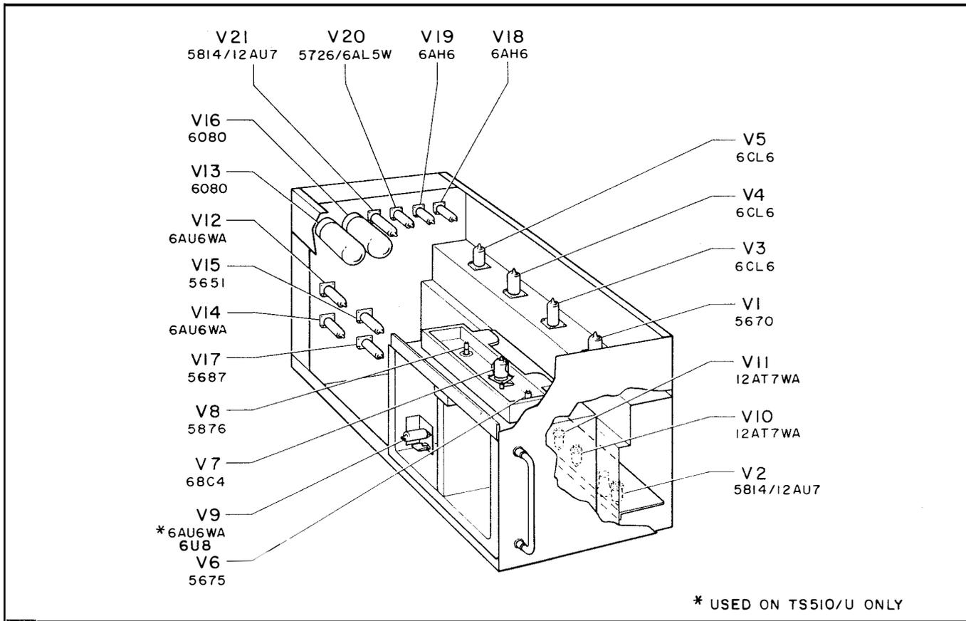
Figure 5-4. Tube Location Diagram
