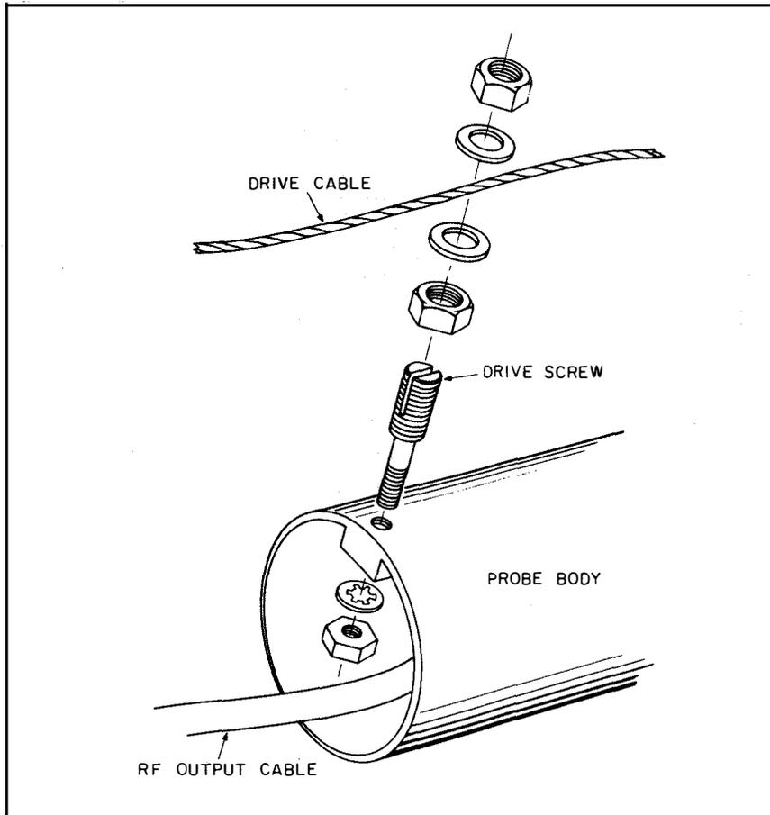
(a) Probe and Cable Attaching Parts
