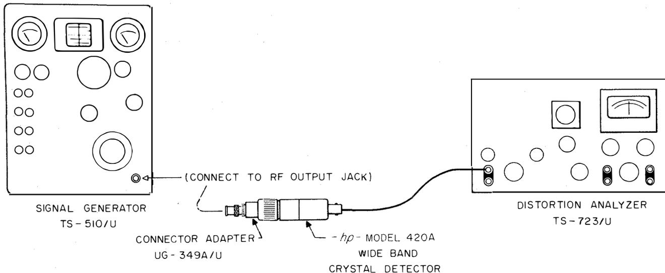
Figure 6-13. Test Set-Up for Measuring the Quality of CW Output Signal
