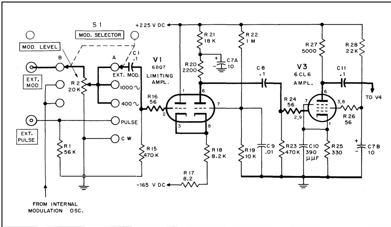
Figure 4-9. Schematic Diagram of Modulation Limiter and Amplifier
