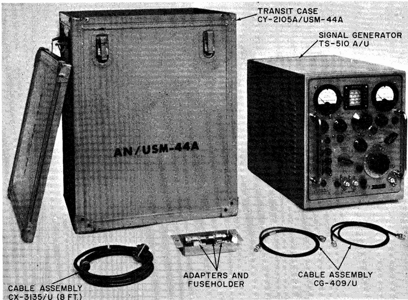
Figure 1-3A. Signal Generator AN/USM-44A (Jetric Industries), Equipment Supplied
