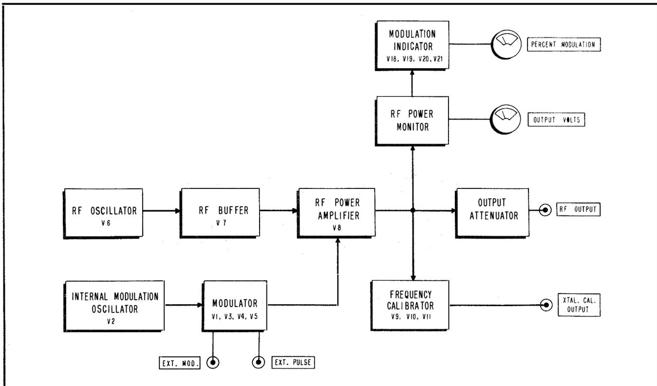
Figure 4-1. Signal Circuit Block Diagram of Signal Generator TS-510A/U
