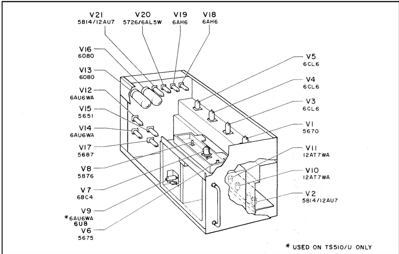
Figure 5-4. Tube Location Diagram
