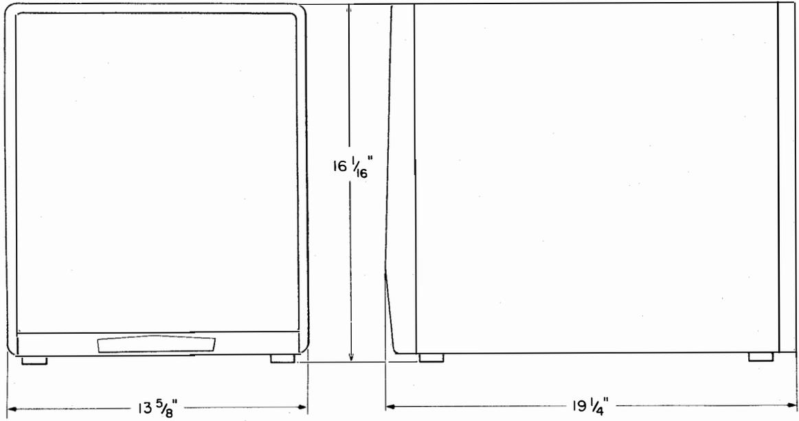
Figure 7-11. Signal Generator TS-510A/U Cabinet Dimensions
