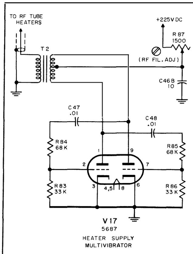
Figure 4-14. Schematic Diagram of Heater Supply Multivibrator
