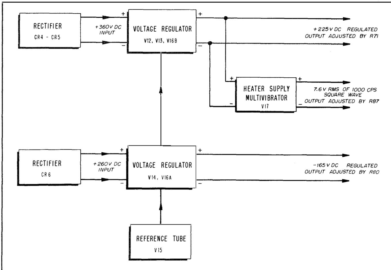
Figure 5-2. Power Supply Block Diagram
