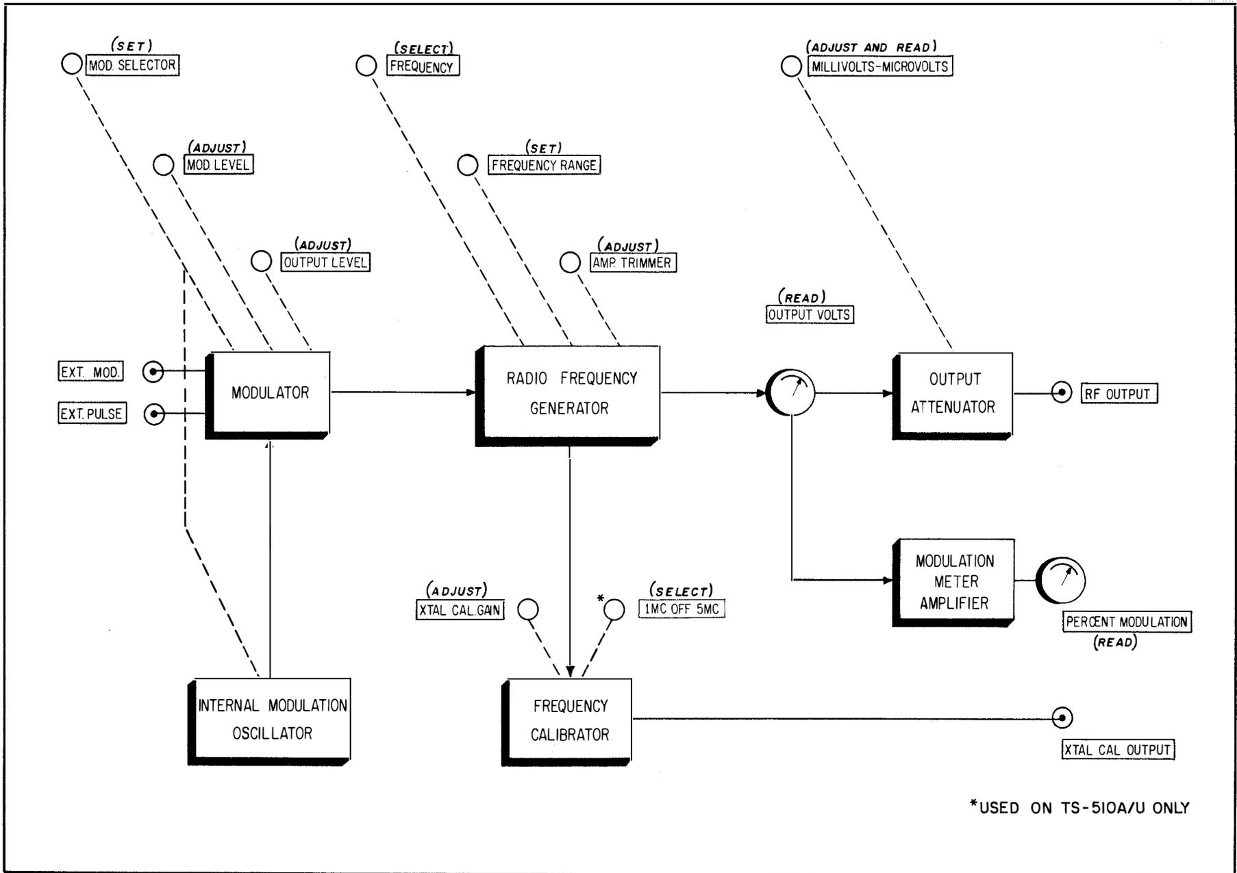
Figure 1-4. Diagram Showing Relationship of Front Panel Controls to Major Circuits
