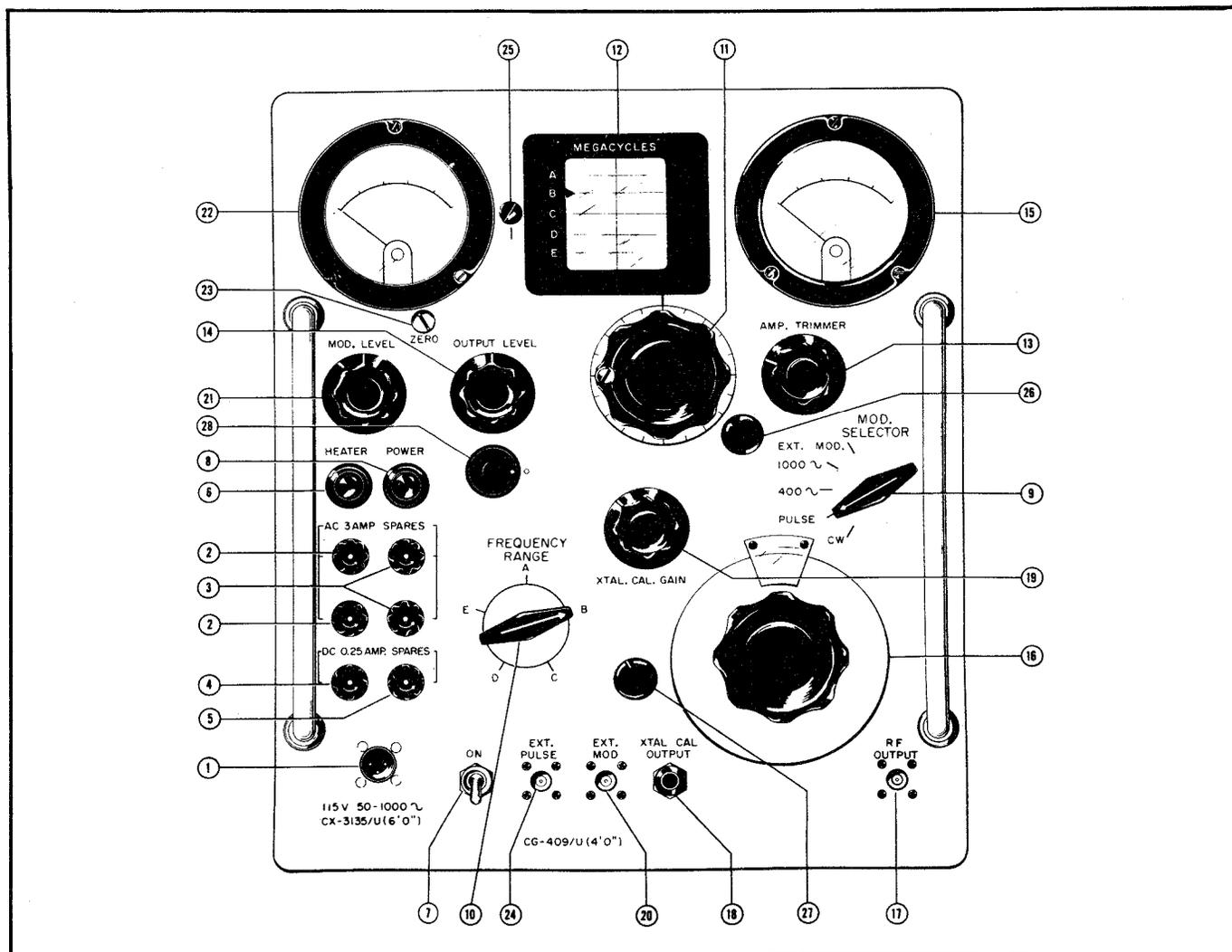
Figure 2-1. Signal Generator TS-510/U (Hewlett-Packard) Front Panel Controls
