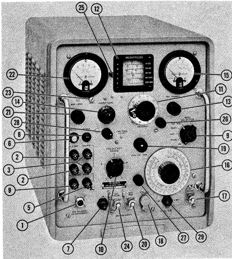
Figure 2-2. Signal Generator TS-510A/U (Hewlett-Packard) Front Panel Controls
