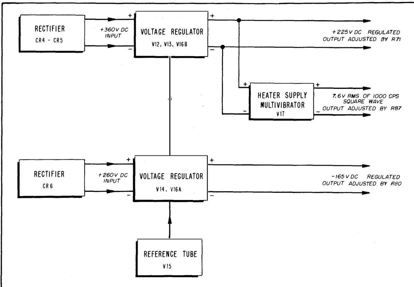
Figure 5-2. Power Supply Block Diagram
