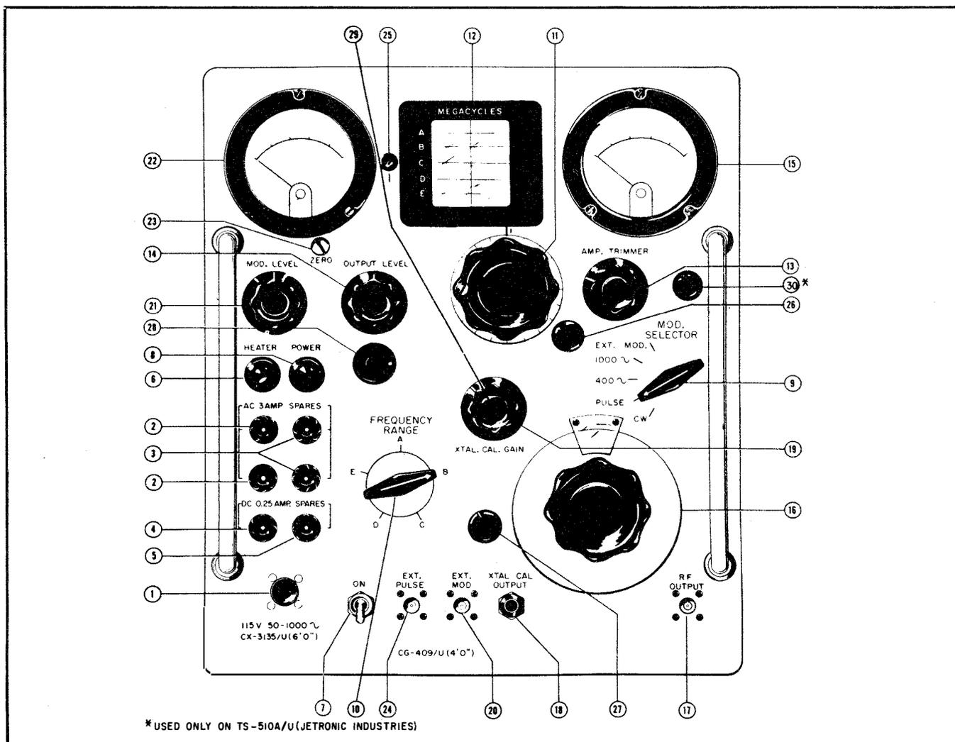
Figure 2-3. Signal Generator TS-510A/U (Nuclear Electronics and Jetronic Industries), Front Panel Controls
