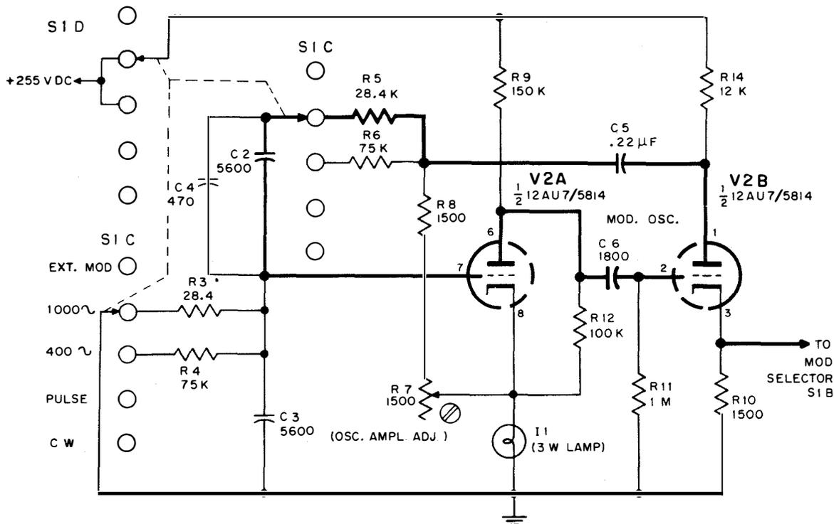
Figure 4-8. Schematic Diagram of Modulation Oscillator
