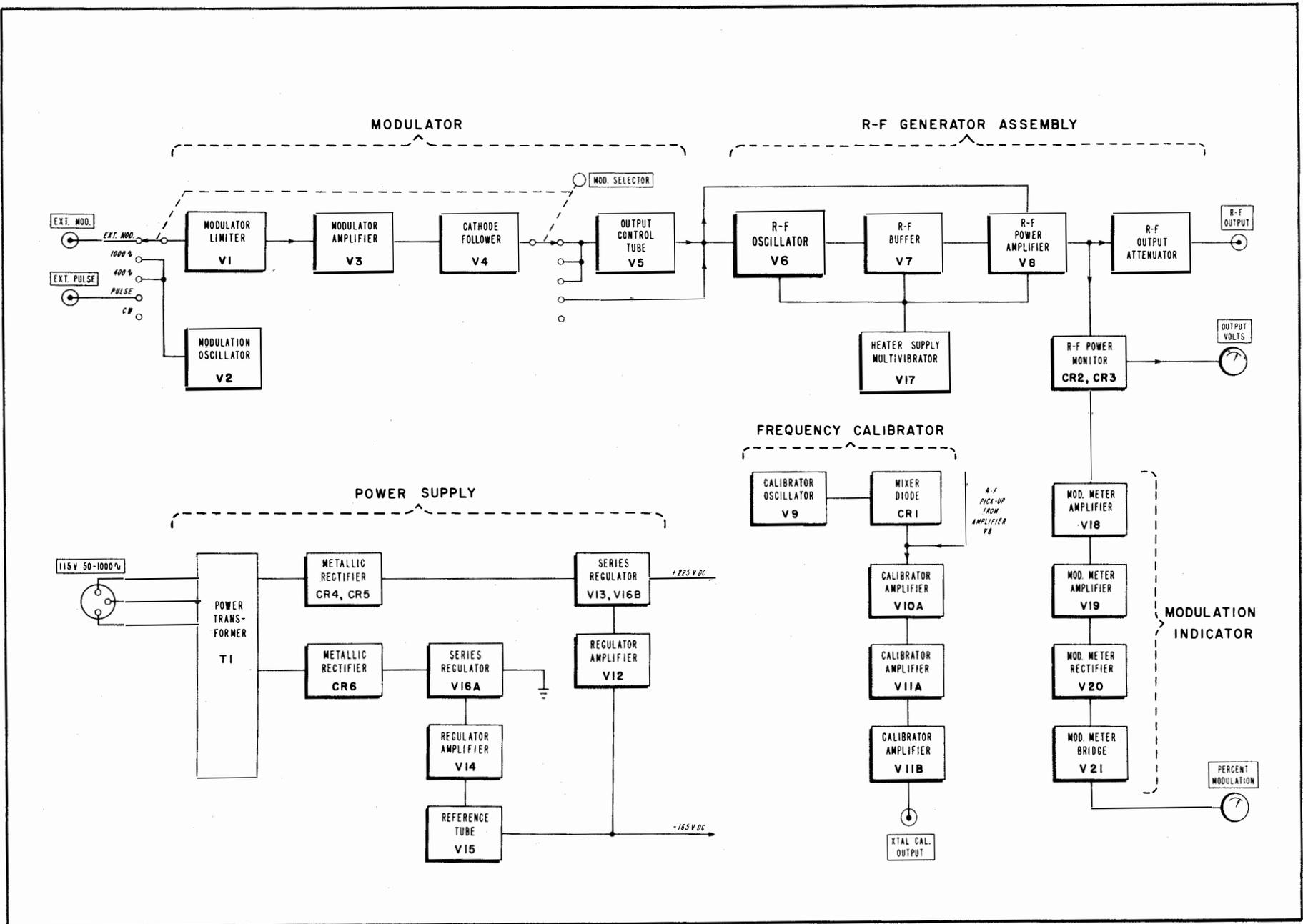
Figure 7-5. Complete Block Diagram for Signal Generator TS-510A/U
