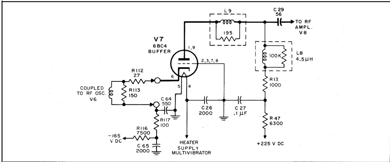
Figure 4-4. Schematic Diagram of Buffer Amplifier
