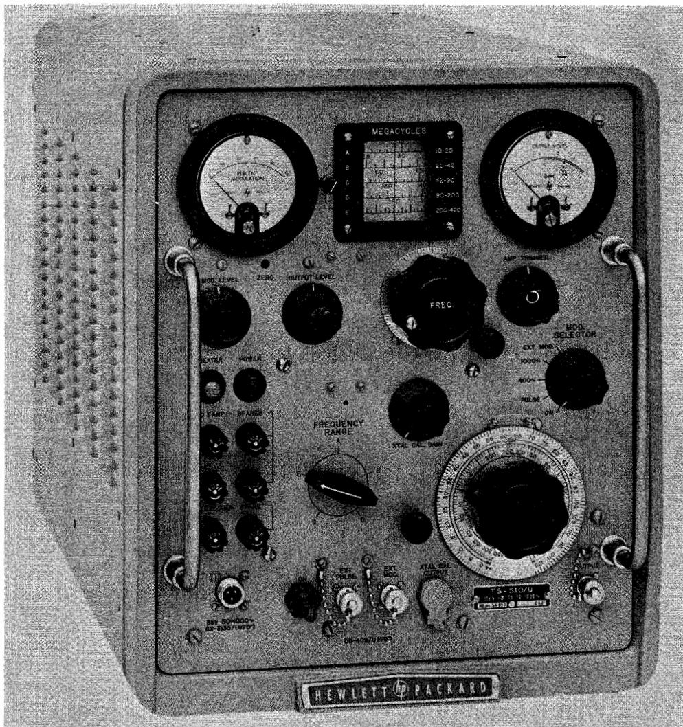
Figure 1-2. Signal Generator TS-510/U
