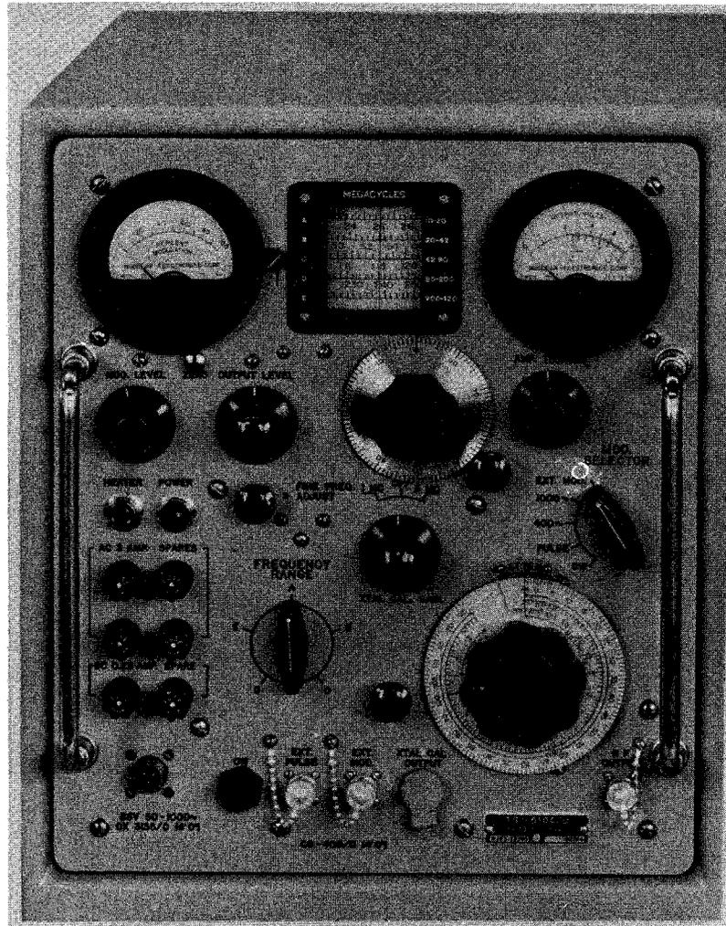
Figure 1-2B. Signal Generator TS-510A/U(\*)
