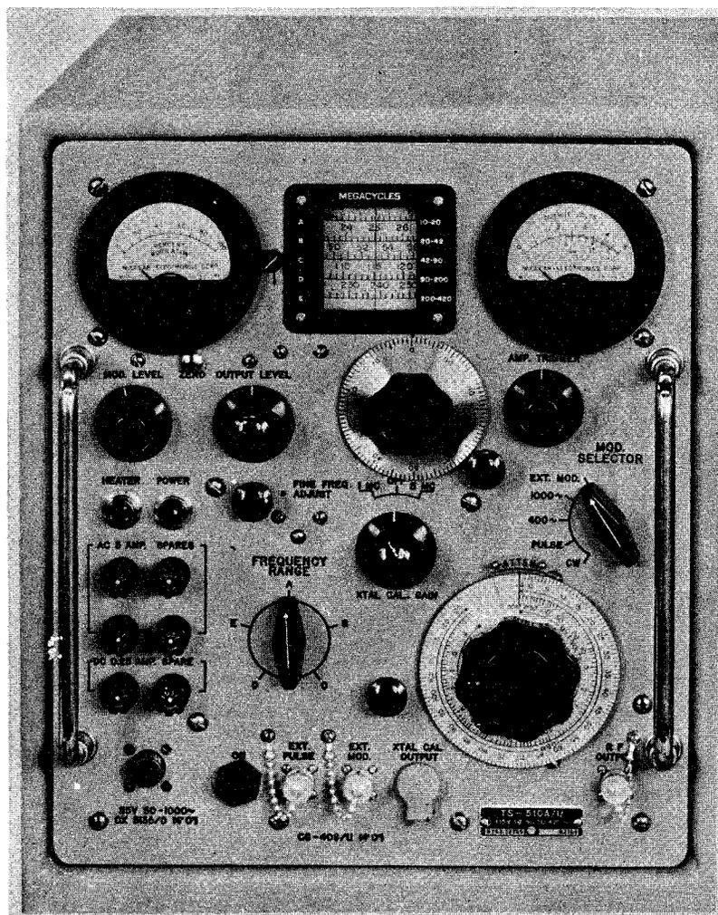
Figure 1-2B. Signal Generator TS-510A/U(\*)
