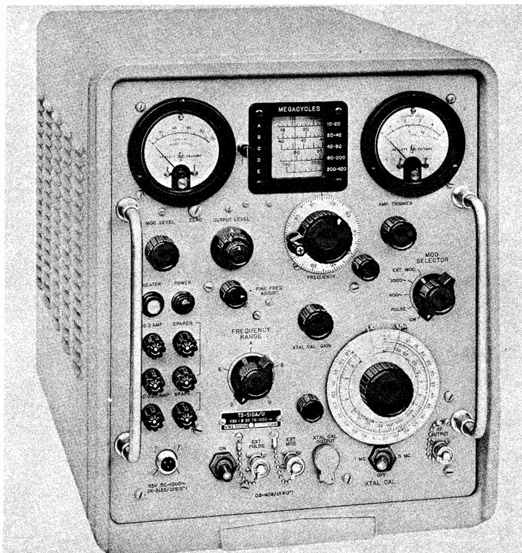
Figure 1-5. Signal Generator TS-510A/U (Hewlett-Packard)
