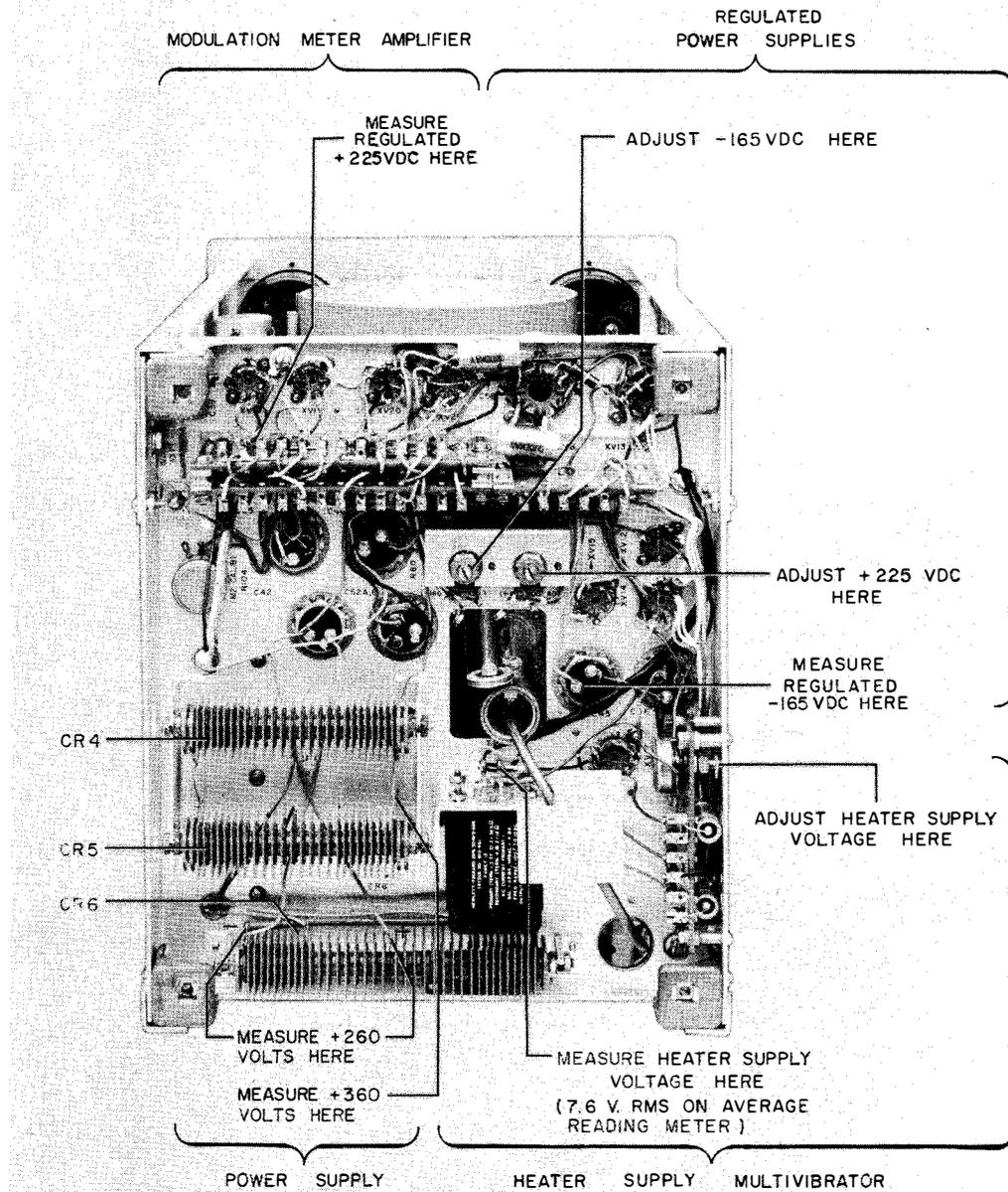
Figure 5-3. Power Supply Section Showing Points of Voltage Measurement and Adjustment
