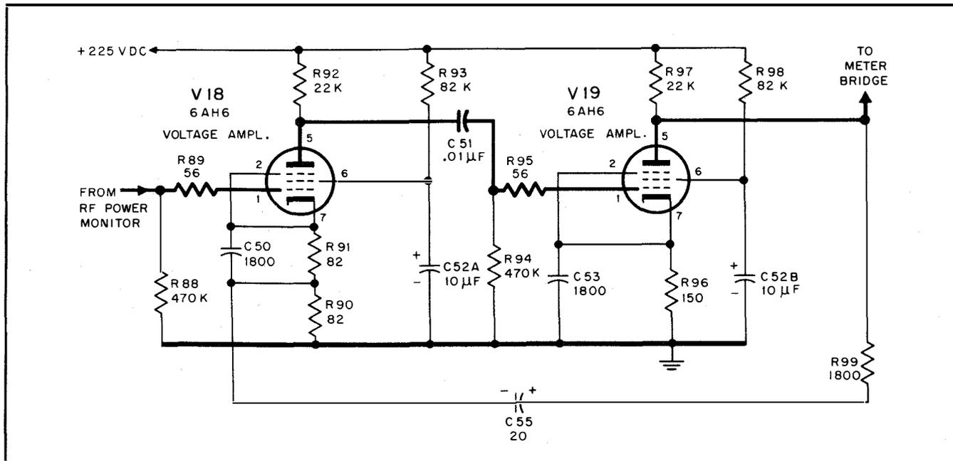
Figure 4-11. Schematic Diagram of Modulation Indicator Amplifier
