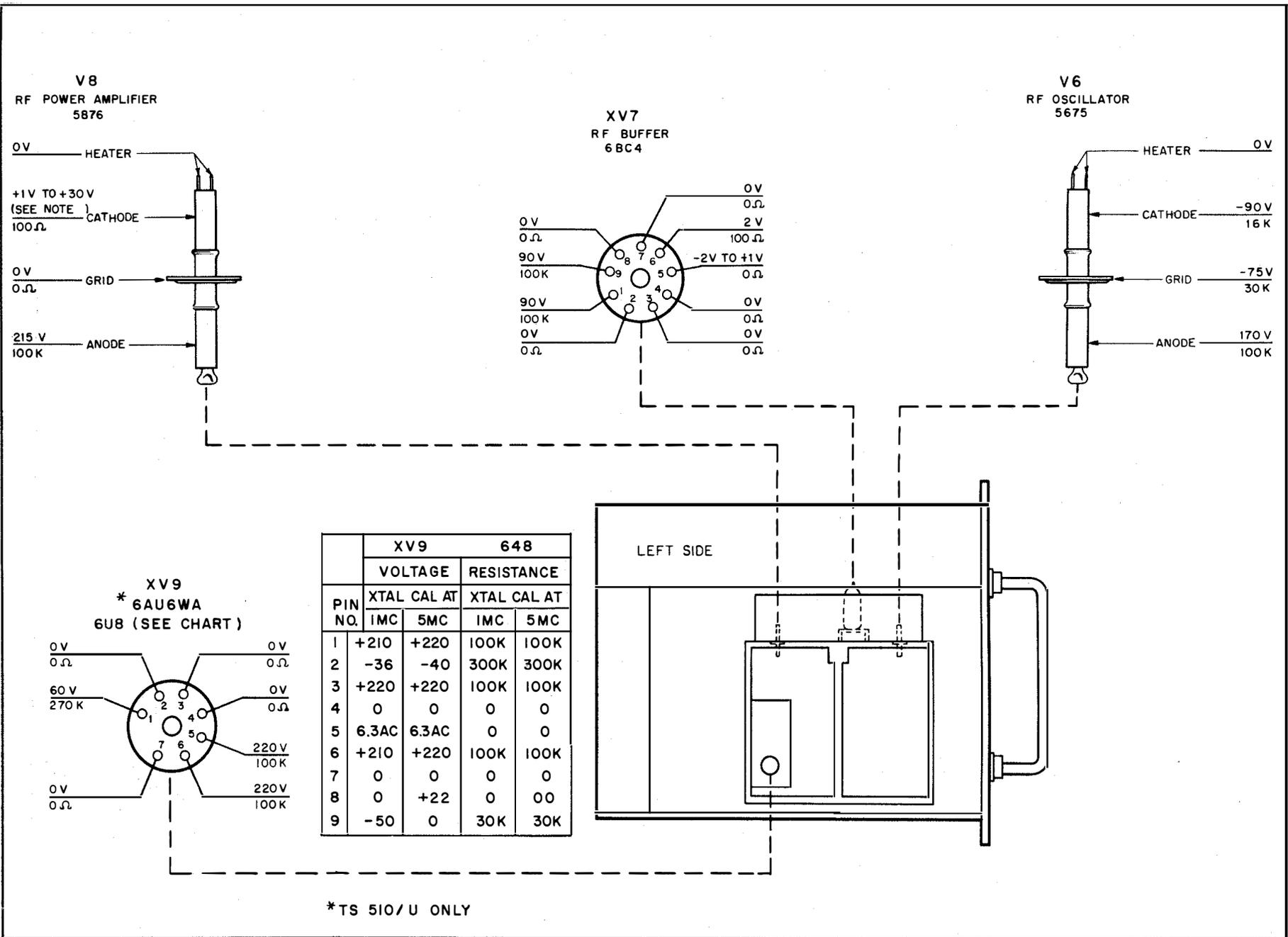
Figure 7-7. Tube Socket Voltage-Resistance Diagram, R-F Generator Section
