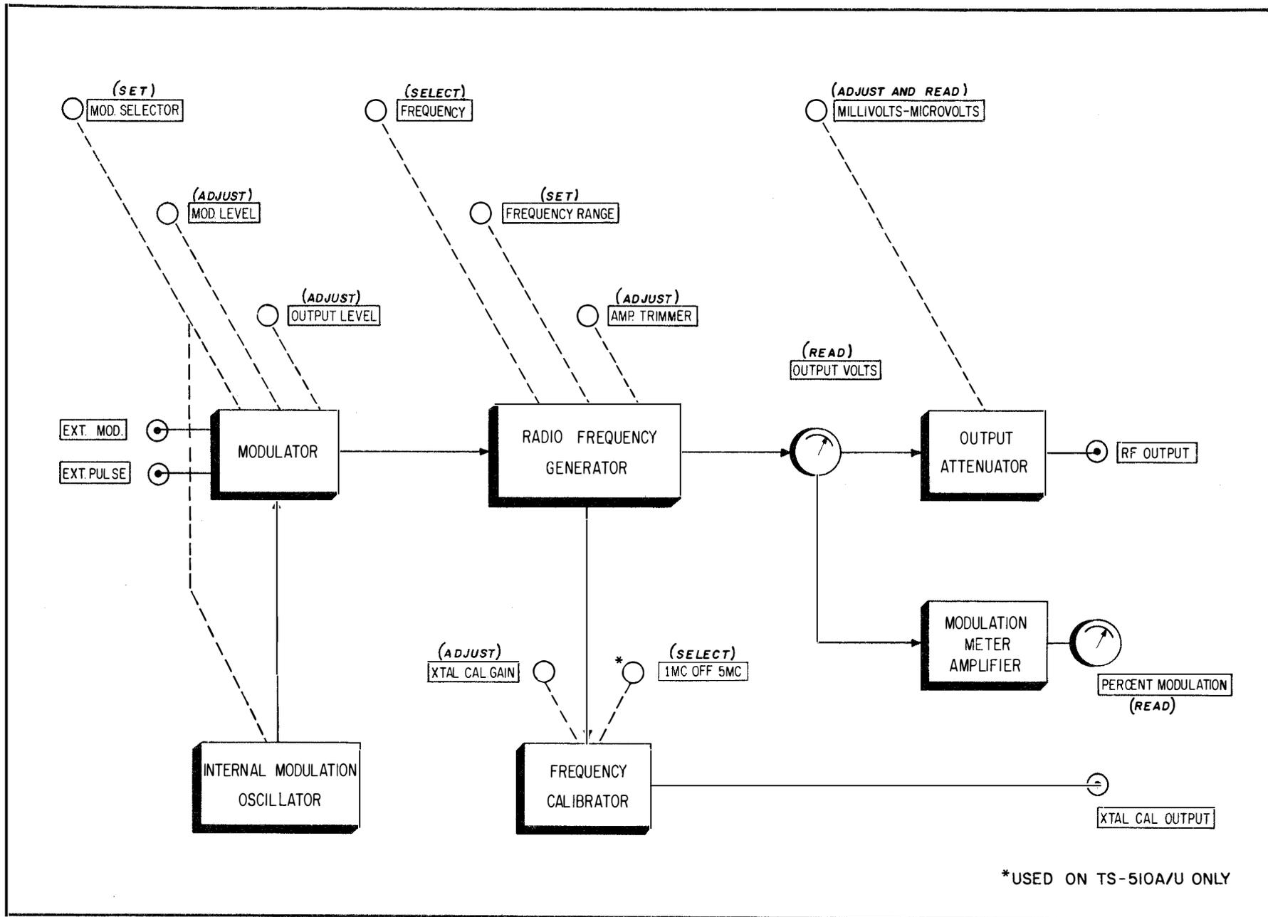
Figure 2-4. Diagram Showing Relationships of Front Panel Controls to Major Circuits
