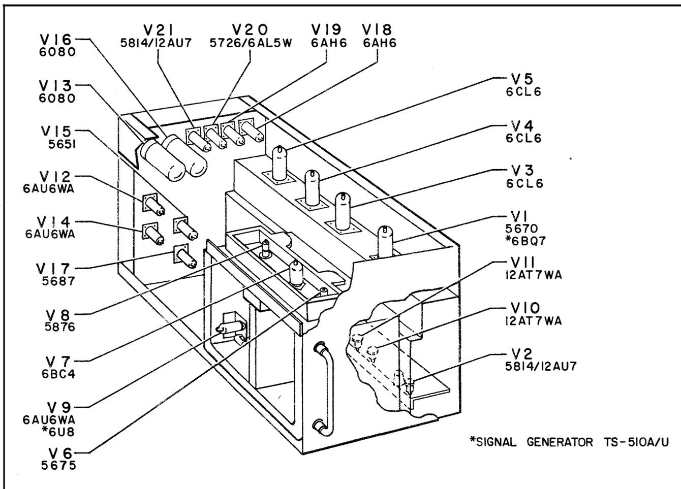
Figure 4-1. Tube Location Diagram
