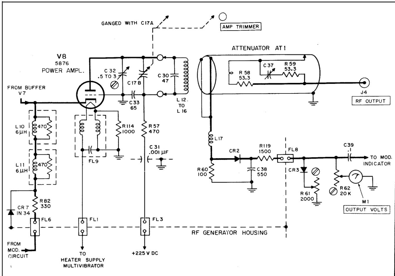
Figure 4-5. Schematic Diagram of Radio Frequency Power Amplifier
