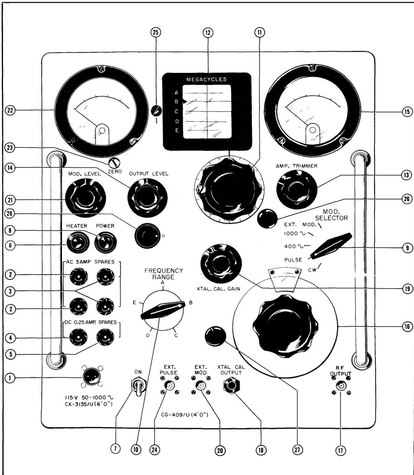
Figure 1-3A. Signal Generator TS-510A/U(\*), Front Panel Controls
