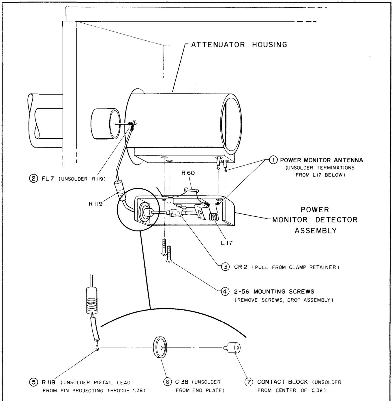
Figure 6-3. Diagram Showing Breakdown of Components in R-F Power Monitor Assembly
