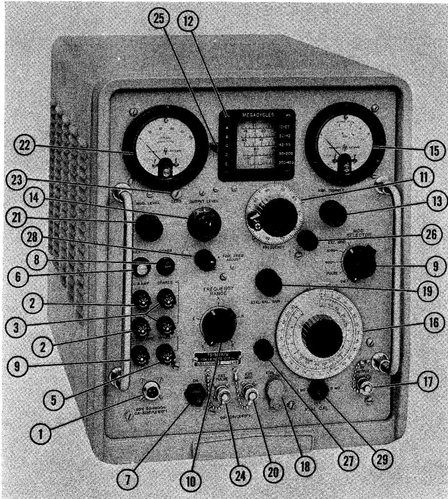
Figure 1-3B. Signal Generator TS-510A/U(\*\*), Front Panel Controls
