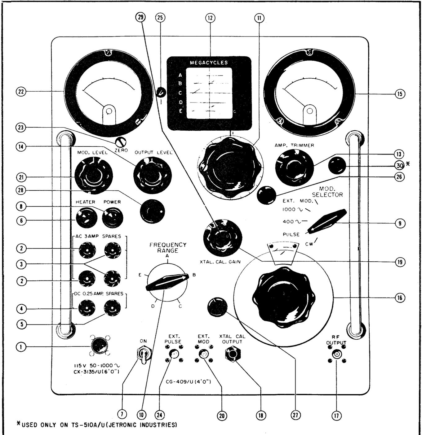
Figure 1-3A. Signal Generator TS-510A/U(\*), Front Panel Controls
