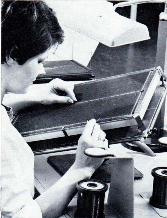
Threading the S-wires of a core-mass memory containing some 130,000 (30 mil) cores.
