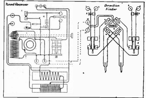
The installation necessary for wireless direction-finding consists of two parts—the aerial circuit and the detecting circuits. The aerial comprises two triangular loops of equal size similarly supported in vertical planes crossing each other at right angles. The loops are usually supported by one corner and are installed with their planes at 45 degrees with the center line of the ship.
