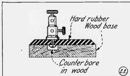
same size as the rubber base but about 1/4 inch thick, is procured and holes drilled in it in such a manner that none of the metal parts touch the wood.
