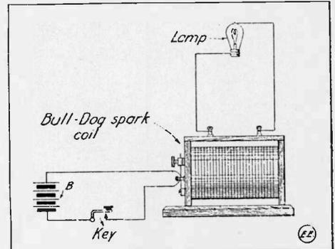
of the globe, but does not have to be. When the current is turned on, a bluish glow will result which resembles the glow of a geissler tube.
