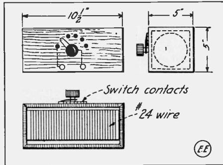
25 cents and taps are brought out at every two inches along the winding and are fastened to the switch contacts as shown. The tube is wound with No. 24 B. & S. single cotton, or enameled magnet wire. The drawings serve to make everything quite clear. This coil in connection with any ordinary receiving transformer will tune to about 3,500 meters.
