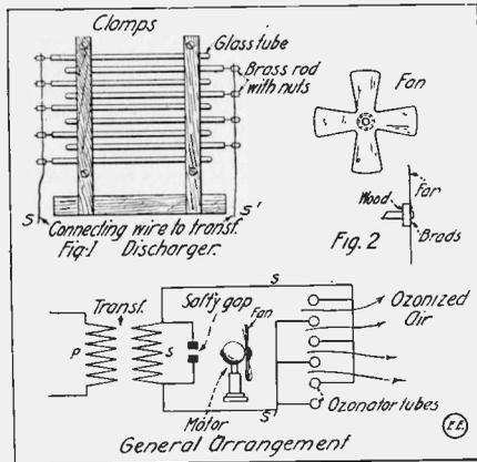
nuts on, toward the right. The next one toward the left, and so on. All rods and tubes are clamped evenly between the clamps as in Fig. 1. (In some case it may be necessary to leave every other glass tube out in order to produce a sufficient amount of ozone.)
