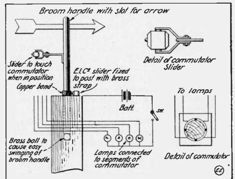
Schematic arrangement of electric weather vane indicator
