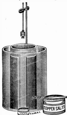
Fig. 2. A Useful Copper Plating Outfit
