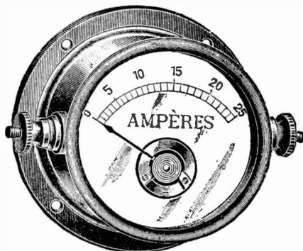
Fig. 9. The Ammeter or Current "Quantity" Gauge
