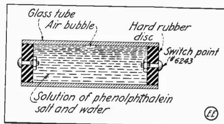
of 3/8" hard rubber to fit tightly into tube. In the exact centre of each piece drill a hole exact size of shank of switch points and mount same on each side.
