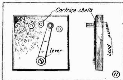
In making small switch boards, I found a good use for old center fire cartridge shells as shown in sketch. A hole a little smaller than the shell is made in the board, then the shell is forced in it. The proper wire is then soldered to one side of the shell or fastened by some means so as to have a good connection.
