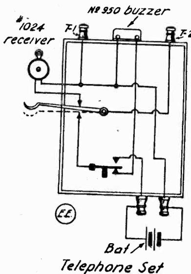
The following articles are needed only to make a two-party telephone that can be used up to a distance of 150 feet or more if E. I. Co. No. 1030 Pony telephone receivers are used instead of No. 1024. The battery used is for signaling purposes only, the receiver being used as a receiver and transmitter both.
