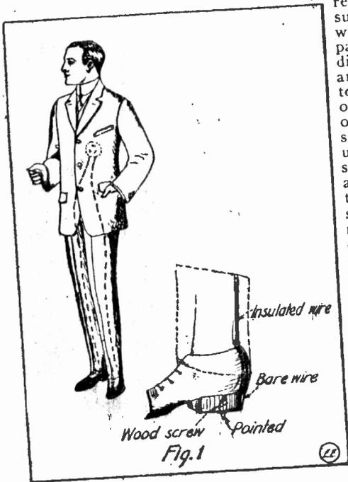
As seen from Figure 1, the detectiphone transmitter and battery perhaps, are placed on an inside coat pocket or a vest pocket, and the two wires leading from same are conducted down underneath the clothes to the heels of the shoes; where, as shown in the detailed sketch, these wires connect with a couple of screws threaded into the heels of the shoes and pointed sharply so that they will readily penetrate an ordinary piece of carpet.
