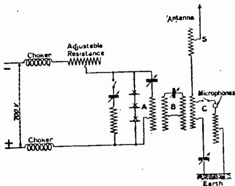
resistance. The voltage at the terminals of the three arcs in series, where the oscillatory circuit is tapped off, is from 250 to 350 volts. When the oscillatory circuit is broken in passing from transmission to reception, this voltage falls to approximately 150 volts, and a resistance is automatically inserted to compensate for this drop in voltage.
