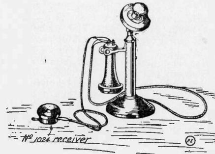
at hand, in the "Electro" No. 1024, 40 cent telephone watch-case receiver, which may be readily connected on multiple to any standard telephone receiver; on any line, as shown in the sketch. A 3-foot double conductor cord, No. 4003 is worth but 15 cents. Many thousands of these auxiliary telephone receivers are
