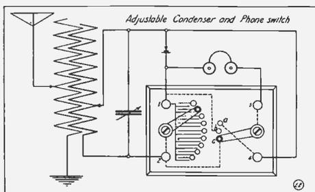
condenser and phone switch make a good combination. A box about three and one-half inches by five inches by one inch, made of hard wood and finished to match the other instruments is used as the container of the condenser and the top
