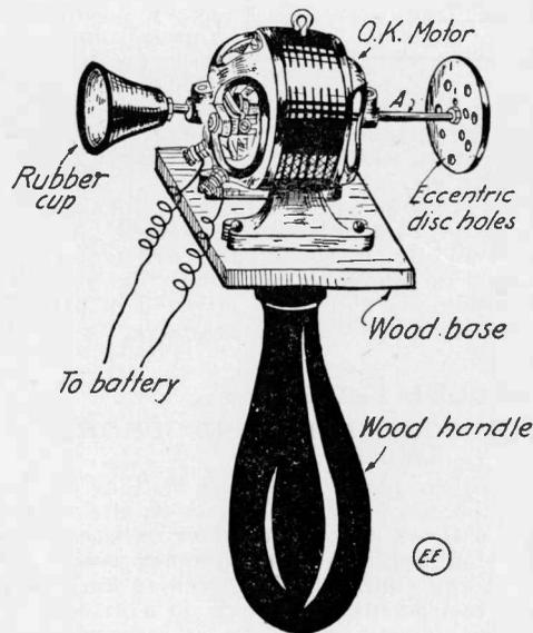
The degree of vibrating massage attained by this machine is governed by a metal disc made of, say  $\frac{1}{8}$  in. brass, and about  $1\frac{1}{2}$  in. diameter. Around this disc is drilled a number of small holes in a spiral or volute path as seen. By placing the shaft thru any desired disc hole, any degree of vibration wanted is readily obtained. The larger the disc and the more eccentric it is placed on the shaft, the greater the vibration produced and vice versa.
