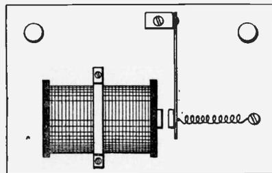
The drawing shows its construction well enough so that a lengthy explanation is unnecessary. An E. I. Co. No. 01107 electro-magnet and some odds and ends, are all the apparatus necessary. The armature is mounted on a piece of
