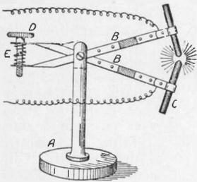
upper end to receive two hinged metal arms B. These are bent to shape at the two rear ends and drilled for the adjustment screw D. This is tapped into the lower arm, the upper one being bored  $\frac{1}{8}$  in. larger to allow of free movement of the screw. The spiral spring keeps them apart until fed together. The front ends are riveted to fibre strips (shown shaded in illustration) to insulate them from the stand and turned into a loop
