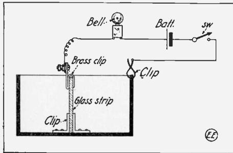
rises that far. Clip one of the E. I. Co.'s helix clips on the edge of the pan. Lead an insulated wire from the bolt on the glass to one of the binding posts of the bell. If there is any slack wire let it hang over the edge of the pan. The diagram of connections is as shown.
