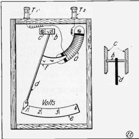
or clock balance wheel setting, or on that principle as detailed in sketch at *c*. The spindle carries a light brass or aluminum wire *d*, which holds the scythe shaped iron armature *f*, and also forms the pointer which moves over the cardboard scale *e*. Cut the armature from the thinnest iron procurable (a condensed milk tin is about right, but if too heavy can be thinned down in dilute nitric acid). It must
