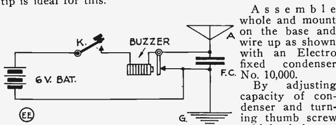
Assemble whole and mount on the base and wire up as shown with an Electro fixed condenser No. 10,000.
