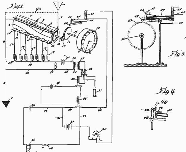
of the coil by gears, 13, 14, so as to rapidly rotate the inductance coil 3.
