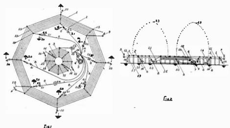
tance above it, as 20 to 25 feet; and thus, this style of antennae is held to be of distinct value; specially as regards the initial cost of erection, which is very great for tall vertical aeriels, having such altitudes as 400 to 800 feet.
