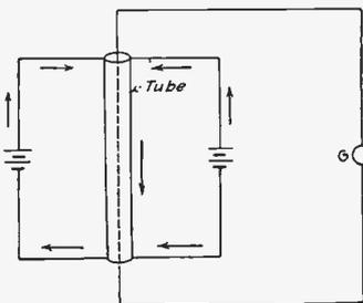
if the tube be threaded with a wire having its ends connected to a galvanometer and the flow of current be interrupted or restored in the tube, an induced E. M. F. will be indicated by the galvanometer, according to Prof. F. J. Rogers, of Princeton University, who submitted this phenomenon to the American Physical Society, at its Washington meeting, as "an electromagnetic puzzle." From his own experiments Professor
