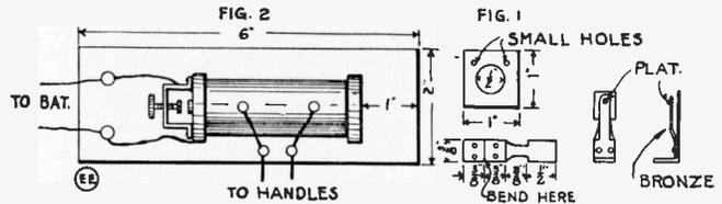
end of No. 24 insulated wire through one of the small holes in the end cheek, and wind on 6 layers; passing the other end thru the second hole in the cheek. Be sure to wind it on smooth.
