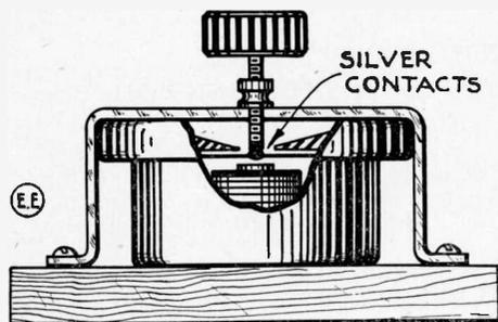
case to the diaphragm and lead the other wire out through the side. Screw the cap on to receiver tightly.
