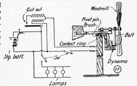
The lights may be used at any time and the dynamo is always charging the battery, whenever its speed is above a certain point, say 1500 to 1600 R. P. M. It is readily geared up to the shaft of the windmill so as to have the proper speed. The battery is, in this case, to be cut off from the dynamo, when it has received full charge; about 2.2 volts per cell on closed circuit, or 1250° Sp. Gr. density in the electrolyte, providing the discharge density value reached about 1150° to 1160° Sp. Gr.
