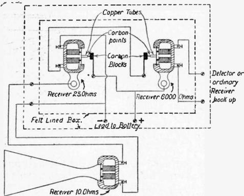
The carbon points against which they rest are made from the lead of an HH pencil. The three telephones are as follows: Firstly, 6,000 ohms; secondly, 25 ohms; and thirdly, about 10 ohms. Up to the present I find that this combination gives me the best results. The weight of the carbon blocks does not seem to be of very great importance, say about 10 grams.
