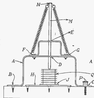
FIG. 1.—DIAGRAMMATIC VIEW OF "QUENCHED" SPARK GAP (EE)
