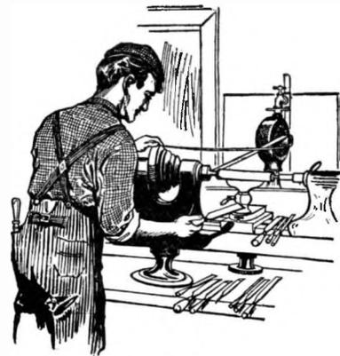
A Lathe Belted Up to the "Hercules" Water Motor.
