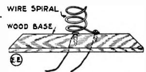
In the center of the block I placed a small flat headed screw which forms a connection with the lamp. Then boring two holes through the block, I inserted two short pieces of flexible wire and soldered one to the screw and the other to the spiral of wire. These I used as terminals for connecting up.
