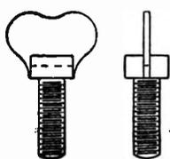
Take a fillister-head screw, measure the thickness of the slot in the head, procure a small piece of sheet steel to make a tight fit in the slot, cut to shape shown in sketch, and drive into head tightly; file up after and polish with emery. This forms an easily-made thumbscrew.—*Model Engineer and Electrician.*
