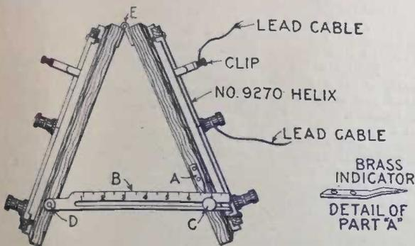
Such a coil, which may be readily employed as a variometer, similar to the Telefunken system, for loading inductance; or as a regular loose-coupling coil for linking the closed condenser and open aerial oscillating circuits, is shown in the sketch here presented.
