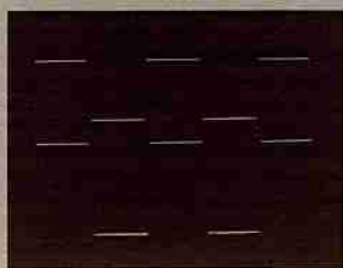
2 KHz Square Wave 150 Watts 8 Ohm Scope: 0.1 msec/cm Top: Input 1.0 v/cm Bottom: Output 20 v/cm
