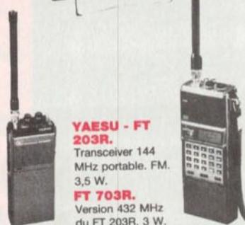
**YAESU - FT 203R.** Transceiver 144 MHz portable. FM. 3,5 W.
