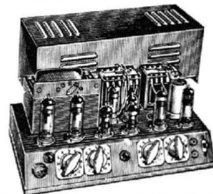
AMPLI VIRTUEUSE PP 30 STEREO 30 WATTS HI-FI 2x15 WATTS
