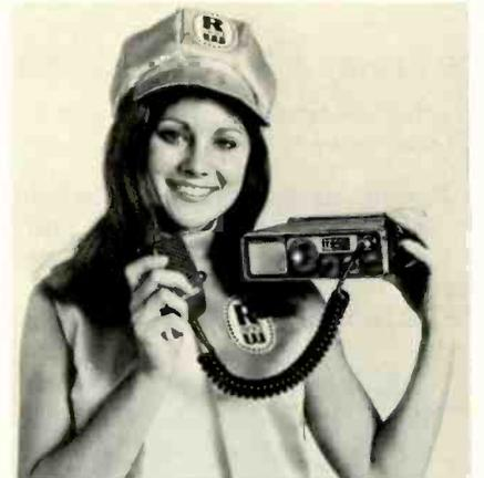
preset to the more commonly used frequencies, but can be reset in the field following the instructions provided with the transceiver. A front panel power selector switch allows a choice of power output of 0.1w, 1.0w or 10w. The power requirement is 13.5v dc  $\pm 10\%$  at 2.42a. The unit has 12 channel capability with a selector switch control. Ross and White Co.
