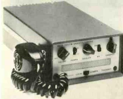
changing. It employs a broadband FET front-end design which provides an average sensitivity of  $0.35\mu\text{v}$  over the entire marine band. Airmarc Corp.
