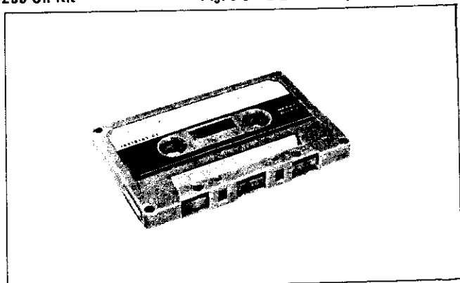
Fig. 3-8 Mirror-equipped Tape Path Test Tape
