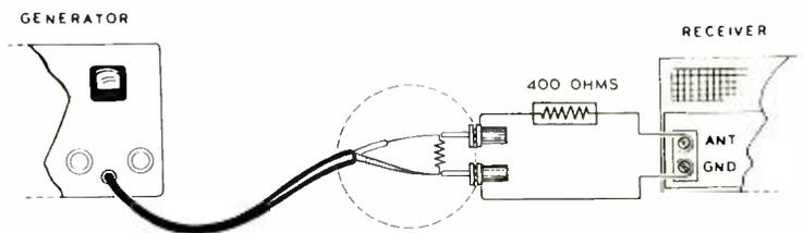
For general test work on all-wave receivers, the I. R. E. (Institute of Radio Engineers) developed a standard dummy antenna. This may be used in place of the 200  $\mu\mu\text{f}$  broadcast dummy and the 400  $\Omega$  shortwave dummy.
