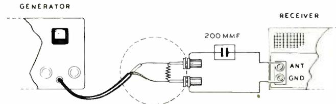
For a short wave receiver, the same type antenna looks like about 400  $\Omega$  resistance.
