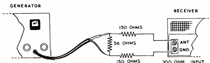
Other circumstances may require the development of different dummy antennas. In the case of IF or stage by stage testing, the signal is generally connected to a grid or plate circuit through a large (.01 to .1  $\mu\text{fd}$ ) condenser. This is done to protect the generator as well as the receiver by keeping the DC voltages from the receiver out of the attenuator and by preventing the attenuator from shorting out the DC operating voltages in the receiver.
