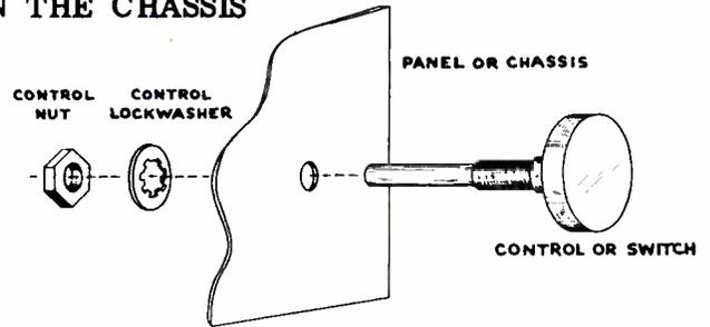
MOUNTING CONTROLS and SWITCHES
