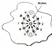
NUMBERING ON 9-PIN TUBE SOCKET
