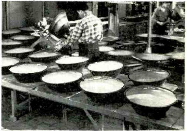
Applying Dixonac coating to inside of funnel and neck of DuMont 19AP4. The dixonac drying conveyor at right of center is in motion. This operation is performed manually.
