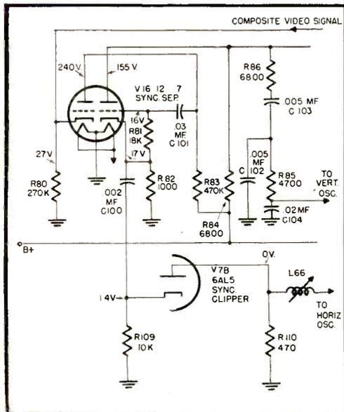
Fig. 4 Duo-triode sync separator and diode sync clipper found in some Motorola sets
