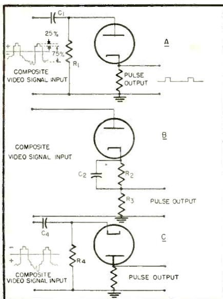
Fig. 1 Three types of diode clippers and the video signals appearing at their inputs
