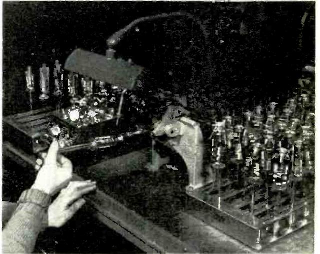
Inspecting cathode and grids. The microscope measures the spacing between cathode and grid. Assembly of the bent electron gun involves such delicate operations that only women are employed in this section of the plant.
