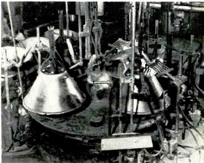
In the pictures that follow, the essential steps in the production of picture tubes are illustrated. At left, one of the first operations is executed: sealing metal cone to glass neck. These tubes are of the short-neck, metal variety. Dr. DuMont foresees larger direct view tubes. He considers a 4 x 5 ft tube very likely.
