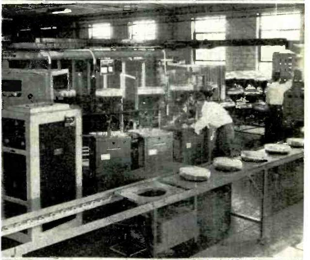
Basing and aging processes at DuMont's Allwood plant. Oven conveyor, on the right, cements base to the neck of the tube. Tubes are aged on conveyor at left while operated at normal potentials.
