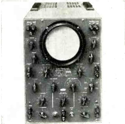
10% from 5 to 200,000 cps. A low voltage version of the instrument is also available as type 250-A. Accelerating potential for the 5CP-A used in this type is 3,000 volts. Detailed information is available from DuMont Labs, Instrument Div., Clifton, N. J.
