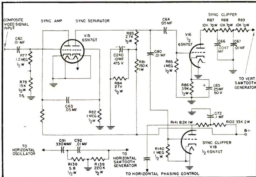
Fig. 5 Four triodes serve as sync amplifier, separator, and clipper (DuMont). This design assures sufficiently high amplitude, freedom from noise and hum
