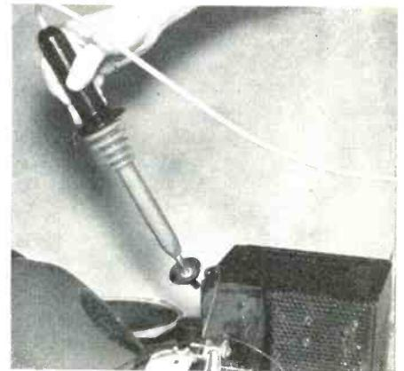
measuring d-c output voltage of pulse-operated and r-f power supplies. For example, if the probe is used with a 100-volt VoltOhmyst meter scale to measure 10,000 volts, the effective resistance of the meter across the voltage source is more than 100,000 ohms per volt deflection. This is especially important where measurement of B plus voltages must be made without loading the circuit. The probes have complete safety features. RCA, Camden, N. J.
