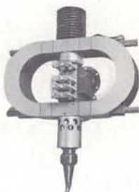
VA-808 Series 5.3 to 5.9 kMc 20 kw peak 300 W average
