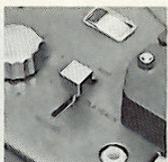
2. Selection of record playback and amplify is accomplished with one knob.
