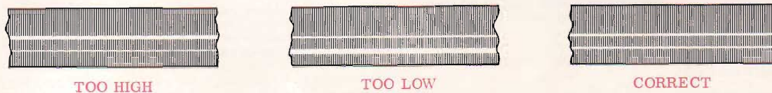
Fig. 3.9 Track measurement, 4-track erase head.
