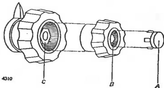
Fig. 15. Removing the knobs
