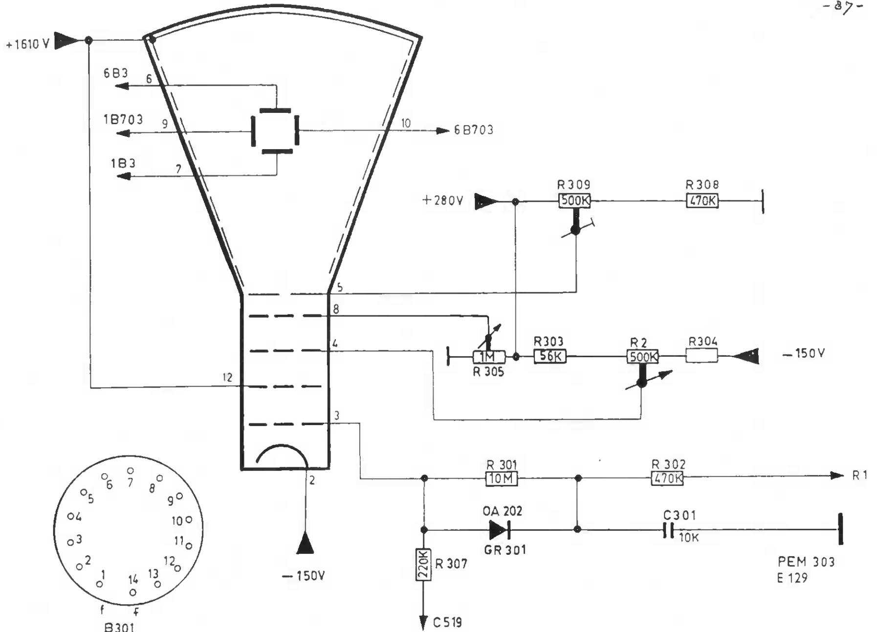
Fig. 35. Diagram of the cathode-ray tube circuit
