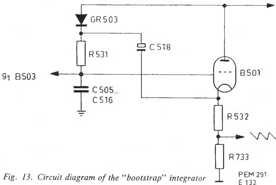
Fig. 13. Circuit diagram of the "bootstrap" integrator
