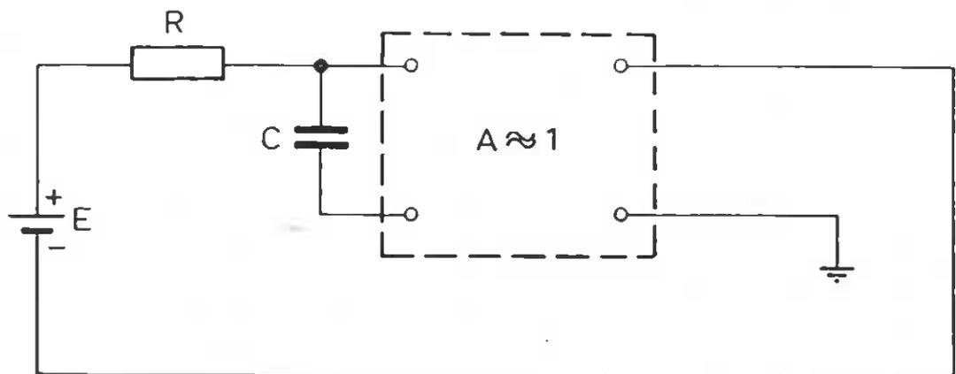
Fig. 12. Block diagram of the "bootstrap" integrator
