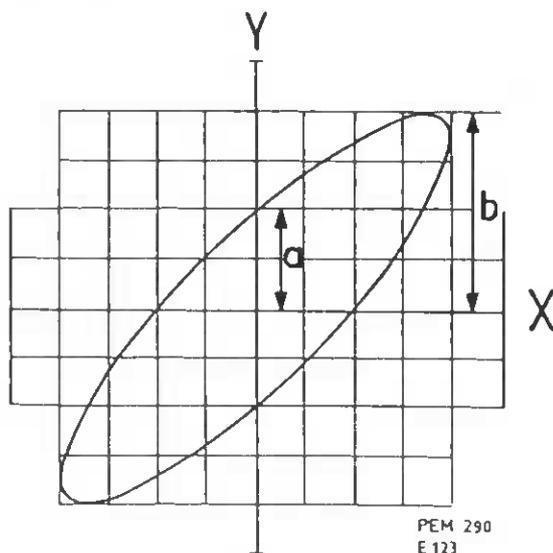
Fig. 7. Determining the phase angles  $\sin \varphi = a/b$
