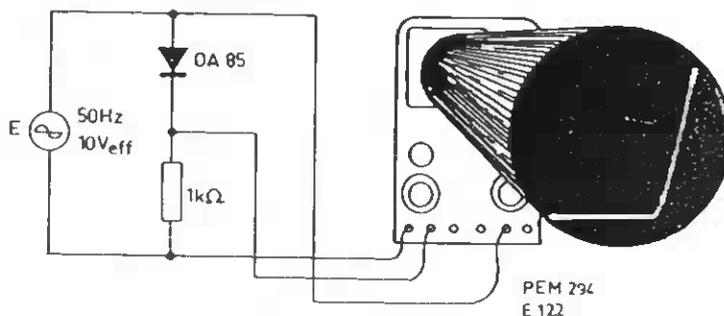
Fig. 10. Displaying the diode characteristic of the 0A 85
