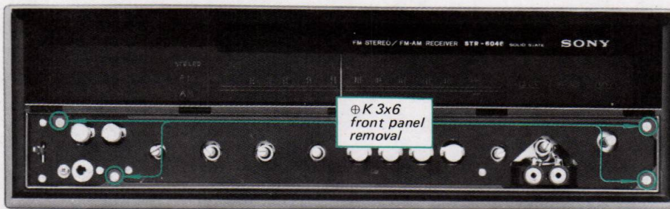
Fig. 2-4. Front panel removal
