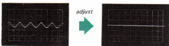
Fig. 3-8. Fm discriminator alignment output response
