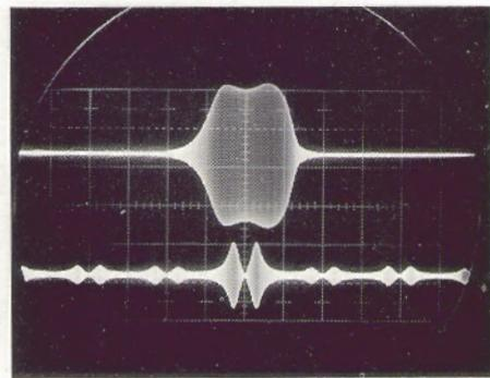
Fig. 3 - WOBULATION D'UN FILTRE A QUARTZ 250 kHz
