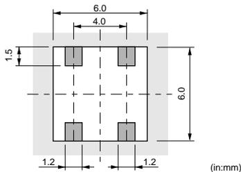
The solder resist should be printed except for the land pattern on the P.C.B.
