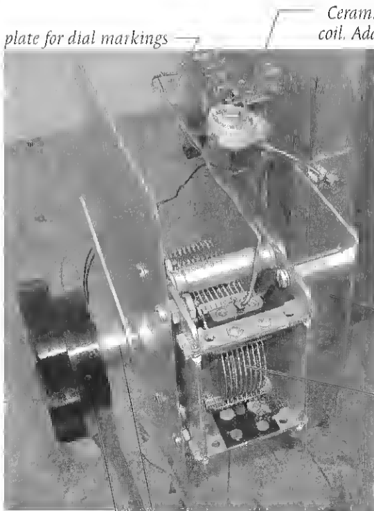
(above) dimension lumber bracket attached to base board (below) details of the tuning capacitor.
