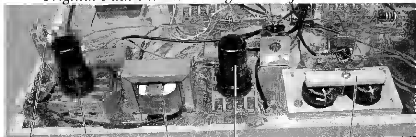
Headphone jack First 6C5 triode 350 H choke Second 6C5 triode Two-pole audio filter on mounted on wood
