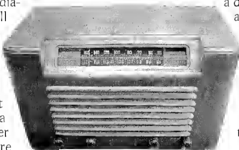
This 1940's vintage shortwave/AM broadcast receiver is equipped with a common slide rule scale dial drive mechanism.
