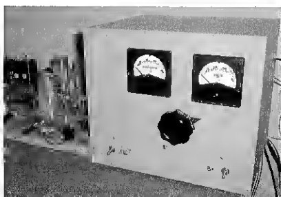
A variac supply that powers an experimental eleven tube superhet receiver (to the left).
