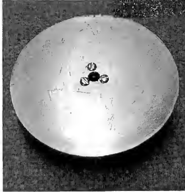
(above) A knob with a large molded-in brass insert was chosen. Holes were drilled and tapped for 4-40 screws. To the right is the final calibrated dial and the hairline plate. (left) the underside of the completed gdo dial
