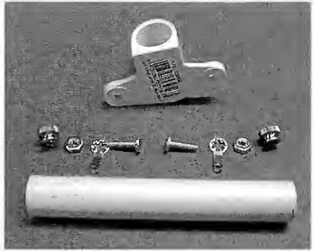
(above) The 1/2" CPVC Wing Elbow and its hardware, and a length of 1/2" CPVC on which the coil will be wound.
