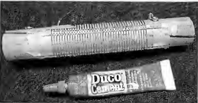
The first bead of cement has been laid.
