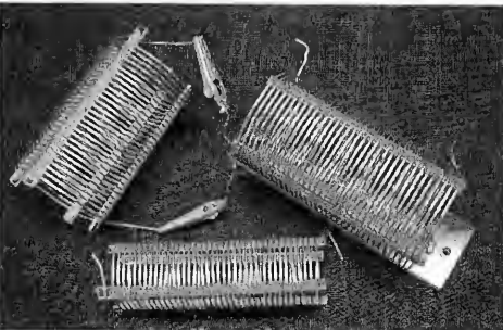
The completed coil is seen at center bottom. The larger coils were wound with a turned mandrel. The coil to the right has been cemented to a section of 1/4" thick acrylic plastic to allow mounting on standoffs.
