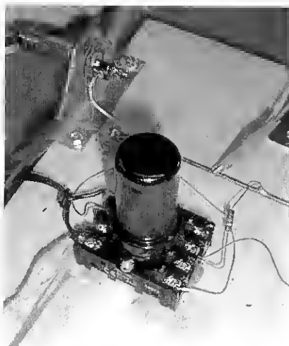
A 6C5 octal metal vacuum tube under test in a plastic relay socket.
