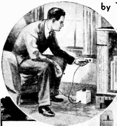
Installation of static-free antenna and line noise filter are shown in above sketches. Mount filter in neatly constructed metal box.
